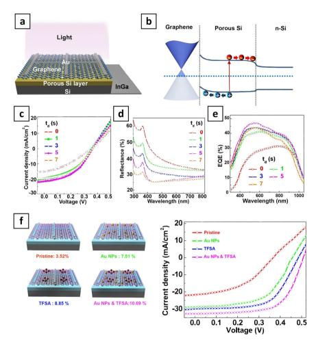
Fig. 13 (a) Schematic illustration of graphene/PSi/n-Si solar cell with Au top contact and InGa bottom contact. (b) Energy band diagrams of the device. (c)–(e) J-V characteristics, reflectance, and EQE spectra of the devices with  $t_d$  from 0 to 7 s. (f) J-V characteristics, and (d) EQE spectra of the pristine, individually doped (Au NPs or TFSA), and co-doped graphene layers/PSi solar cells. Reproduced from ref. 163, with permission from the Royal Society of Chemistry.
