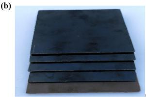
Fig. 1 (a) Schematic fabrication process of carbon nanotube-reinforced stone waste epoxy polymer composite. (b) Carbon nanotube-reinforced composite sheet
