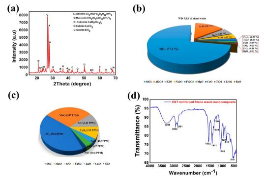
Fig. 2 (a) XRD of CNT-reinforced stone waste polymer nanocomposite. (b and c) XRF results of the stone waste. (d) FTIR of CNT-reinforced stone waste polymer nanocomposite.
