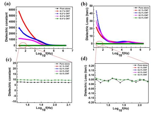
Fig. 6 (a) Dielectric constant. (b) Dielectric loss of pristine and CNT reinforced stone waste nanocomposite samples. (c) Enlarged view of the dielectric constant and (d) enlarged view of the dielectric loss of pristine and CNT reinforced stone waste nanocomposite samples
