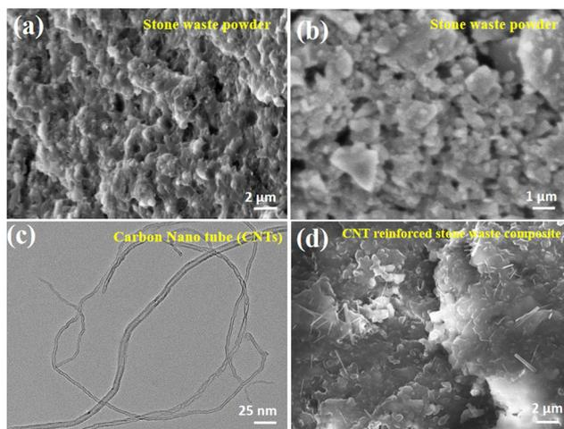
Fig. 3 (a and b) SEM image of the stone waste powder sample. (c) TEM image of the CNT and (d) stone waste polymer nanocomposite sample.
