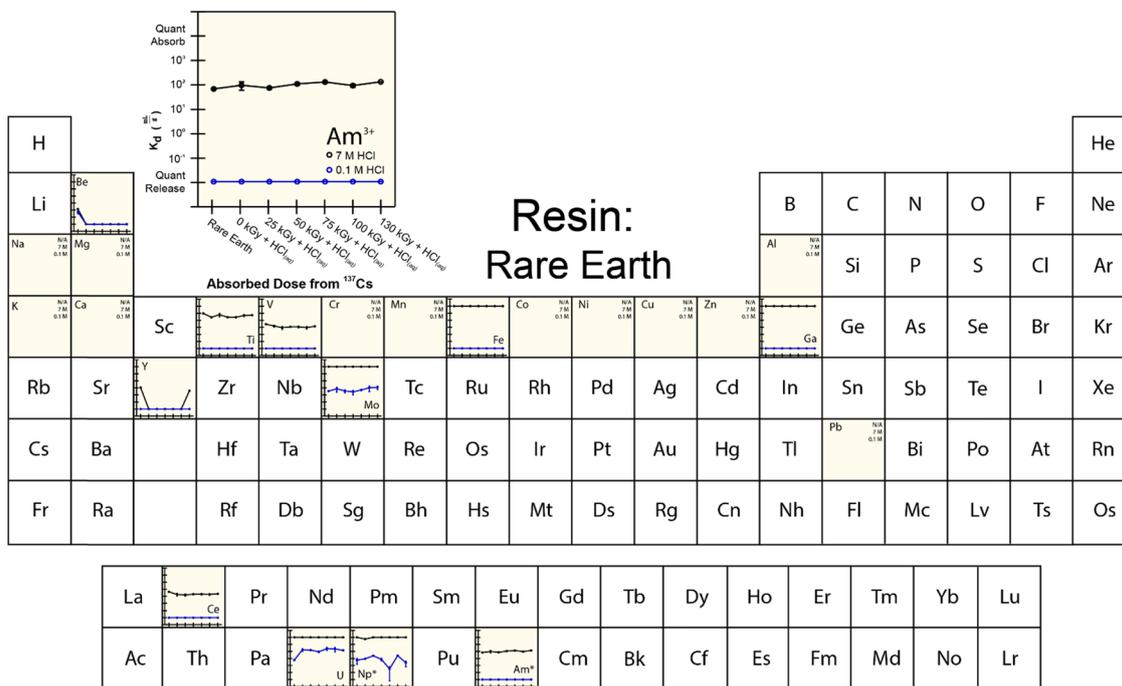
Fig. 5 Temperature controlled (25 °C) distribution coefficients ( $K_d$ ) from Rare Earth (RE) resin for  $^{241}\text{Am}_{(\text{aq})}$  (20 pCi) in HCl (0.1 and 7 M) with twenty-three metal contaminants present at 5 ppm. Measurements were made in triplicate and uncertainty is shown as the standard deviation of the mean (at  $1\sigma$ ). Elements labeled with N/A were not adsorbed. The asterisk (\*) indicates when analytes were present on a microscopic scale and used as a radiotracer.
