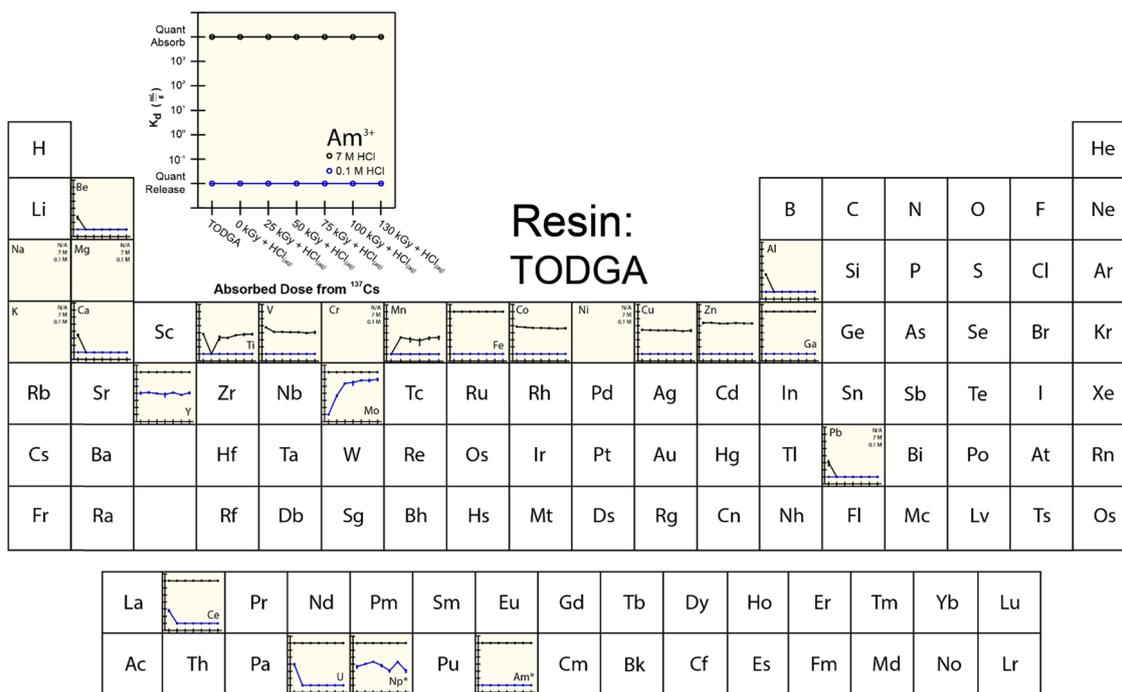
Fig. 6 Temperature controlled (25 °C) distribution coefficients ( $K_d$ ) from TODGA resin for  $^{241}\text{Am}_{(\text{aq})}$  (20 pCi) in HCl (0.1 and 7 M) with twenty-three metal contaminants present at 5 ppm. Measurements were made in triplicate and uncertainty is shown as the standard deviation of the mean (at  $1\sigma$ ). Elements labeled with N/A were not adsorbed. The asterisk (\*) indicates when analytes were present on a microscopic scale and used as a radiotracer.
