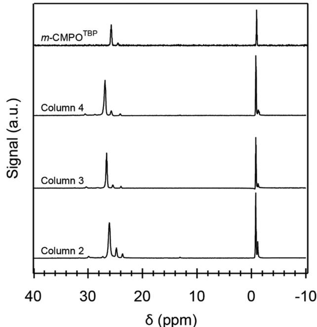
Fig. 10 The  $^{31}\text{P}$  NMR ( $^1\text{H}$ -coupled) spectra from 'pristine'  $m\text{-CMPO}^{\text{TBP}}$  resin (top, no  $^{241}\text{Am}$  nor acid exposure) and resin aliquots taken from active columns (2, 3, and 4) used in the CLEAR process ('veteran' resin samples that were exposed to acid and  $^{241}\text{Am}$ ). The  $^{241}\text{Am}$  radiation dose received by the veteran resin decreased from Column #2 to Column #4. Data was normalized to  $m\text{-CMPO}$  at  $\delta$  26 ppm.
