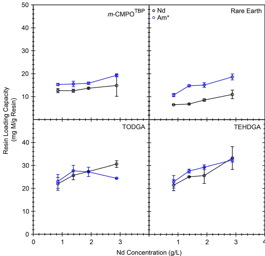
Fig. 9 Temperature controlled (25 °C) Nd<sup>3+</sup>/Am<sup>3+</sup> loading capacity as a function of Nd concentration with HCl<sub>(aq)</sub> held at a constant initial concentration of 7 M. The asterisk (\*) indicates when analytes were present on a microscopic scale and used as a radiotracer.
