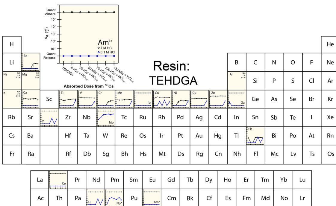
Fig. 7 Temperature controlled (25 °C) distribution coefficients ( $K_d$ ) from TEHDGA resin for  $^{241}\text{Am}_{(\text{aq})}$  (20 pCi) in HCl (0.1 and 7 M) with twenty-three metal contaminants present at 5 ppm. Measurements were made in triplicate and uncertainty is shown as the standard deviation of the mean (at  $1\sigma$ ). Elements labeled with N/A were not adsorbed. The asterisk (\*) indicates when analytes were present on a microscopic scale and used as a radiotracer.
