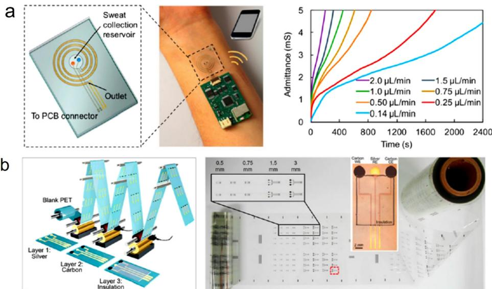
Fig. 7 (a) Microfluidics-based sensing system for sweat sampling, sensing, and sweat rate analysis. Reprinted with permission, Copyright,<sup>109</sup> 2018 American Chemical Society. (b) Roll-to-roll gravure printing enabled mass production of high-performance flexible chemical sensors at low cost. Reproduced from ref.110 Copyright 2018 American Chemical Society.
