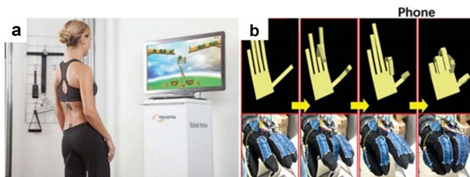
Fig. 11 (a) Motion-sensing game with a wearable stress sensor system<sup>162</sup> (reprinted with permission Copyright 2012, BioMed Central). (b) The capture and digitalization of hand motion with a smart glove integrated with sensors.<sup>163</sup> (Reprinted with permission Copyright 2014, American Chemical Society).
