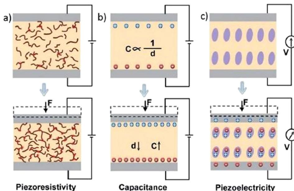
Fig. 5 Schematic illustrations<sup>109</sup> of transduction methods: (a) piezoresistivity, (b) capacitance, and (c) piezoelectricity. (Adapted and reprinted with permission, Copyright 2015, Royal Society of Chemistry).
