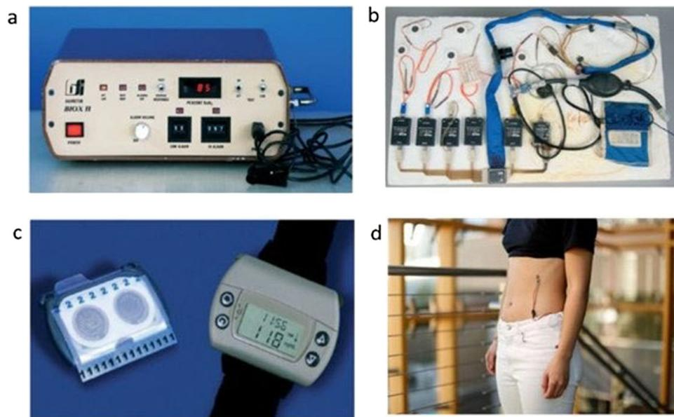
Fig. 2 Some historical glimpses of wearable sensors: (a) pulse oximetry for wearing on the fingertip, (b) wearable sensors used during the Apollo Space Program, (c) an early wearable digital glucose sensor for diabetic patients, and (d) 'Sport Tester PE2000' heart rate monitor by Polar. (Adapted and reprinted with permissions,<sup>35</sup> Copyright 2018, Royal Society of Chemistry).
