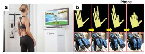
Fig. 11 (a) Motion-sensing game with a wearable stress sensor system<sup>162</sup> (reprinted with permission Copyright 2012, BioMed Central). (b) The capture and digitalization of hand motion with a smart glove integrated with sensors. 163 (Reprinted with permission Copyright 2014, American Chemical Society).
