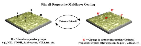
Fig. 2 Schematic representation of the stimuli-responsive coating/film with dynamic liquid wettability.
