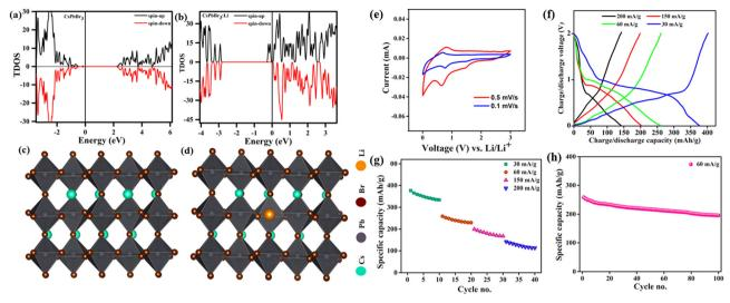
Fig. 2 TDOS of CsPbBr<sub>3</sub> without (a) and with Li<sup>+</sup> (b). Side views (c and d). CV curves (e), GCD curves (f), specific discharge capacity (g), and cycling diagram (h) of CsPbBr<sub>3</sub>. 48 Copyright © 2021 American Chemical Society.
