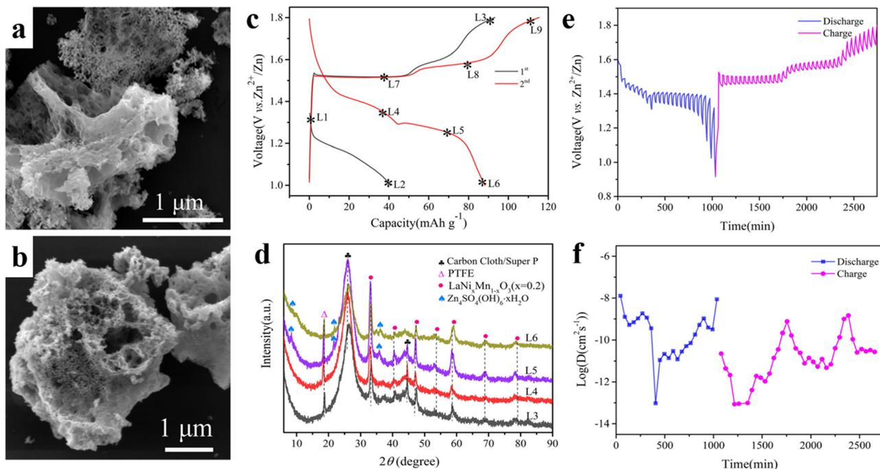
Fig. 11 SEM of  $\text{LaNi}_x\text{Mn}_{1-x}\text{O}_3$  ( $x = 0.2$ ) (a) and  $\text{LaMnO}_3$  (b). Charge/discharge curves (c), XRD at different voltages (d), GITT curves (e) and diffusion coefficients (f) of  $\text{LaNi}_x\text{Mn}_{1-x}\text{O}_3$  ( $x = 0.2$ ).<sup>120</sup> Copyright © 2022 Elsevier.
