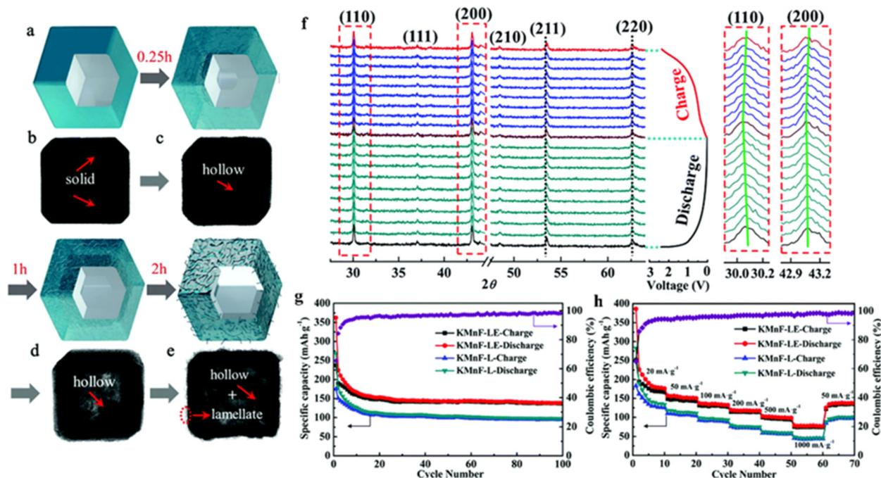
Fig. 10 Synthesis and characterization of hollow KMnF-LE (a–e). *In situ* XRD patterns of KMnF-LE (f). Cyclic stability (g) and rate performance (h) of KMnF-L and KMnF-LE.<sup>113</sup> Copyright © 2018 Royal Society of Chemistry.
