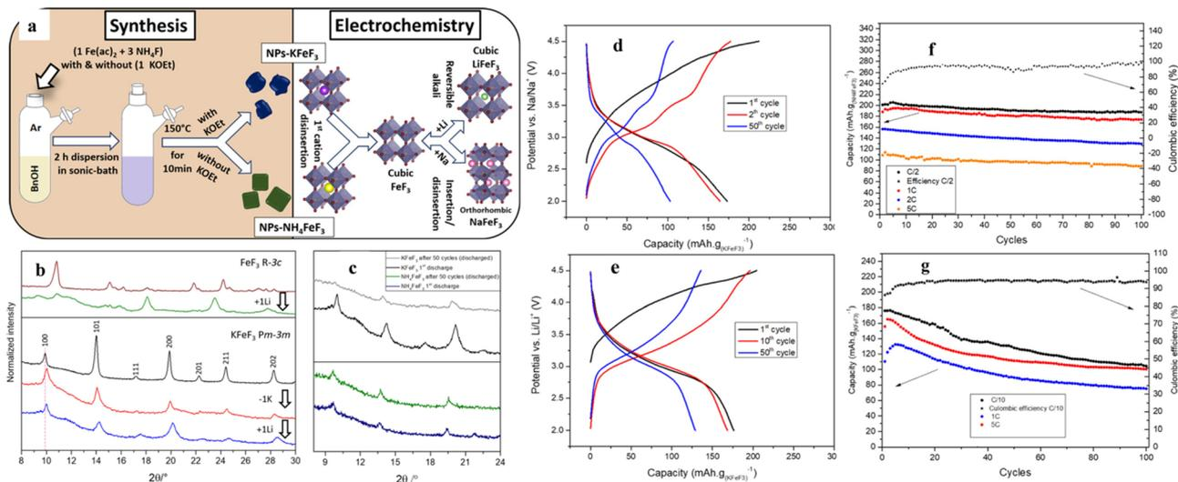
Fig. 4 Synthesis roadmap and model diagram of  $\text{K}/\text{NH}_4^+\text{FeF}_3$  (a). *Ex situ* XRD of  $\text{KFeF}_3$  during charging and discharging (b). Comparison of *ex situ* XRD of  $\text{NH}_4\text{FeF}_3$  and  $\text{KFeF}_3$  (c). GCD of  $\text{NH}_4\text{FeF}_3$  at C/10 (d) and  $\text{KFeF}_3$  at C/2 (e) toward Li. Cycling performance of  $\text{NH}_4^+\text{FeF}_3$  (f) and  $\text{KFeF}_3$  (g).<sup>65</sup> Copyright © 2019 American Chemical Society.
