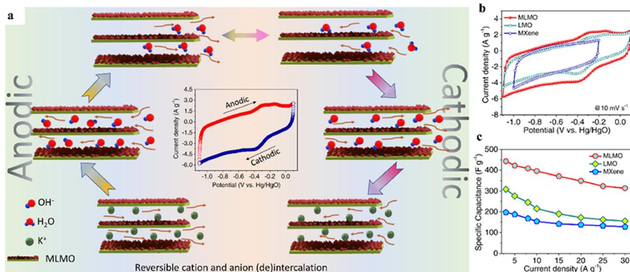
Fig. 14 Schematic illustration of reversible cation and anion (de)intercalation in MLMO (a). Comparison of CV curves (b) and specific capacitances (c) of LMO, MXene and MLMO.<sup>152</sup> Copyright © 2022 Elsevier.
