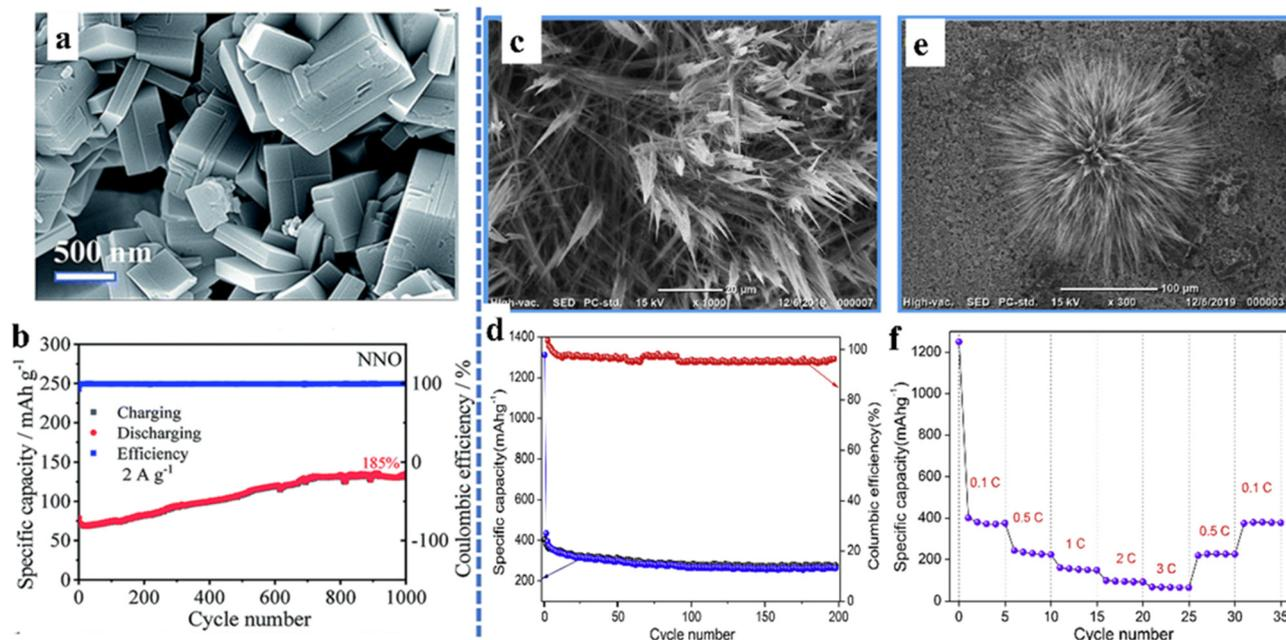
Fig. 6 SEM micrograph (a) and cycling performance (b) of  $\text{NaNbO}_3$ .<sup>81</sup> Copyright © 2019 Royal Society of Chemistry. SEM micrographs (c and e), cycling performance (d) and rate performance (f) of nanostructured flowerlike  $\text{KTaO}_3$ .<sup>82</sup> Copyright © 2019 Elsevier.
