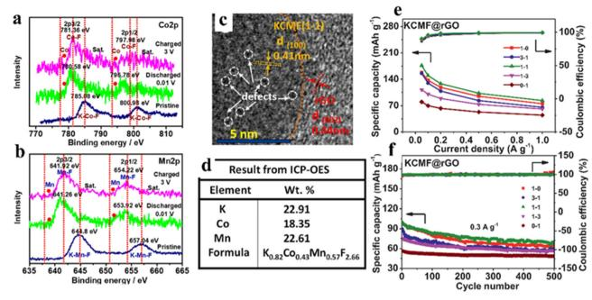
Fig. 8 Co2p (a) and Mn2p (b) of KCMF(1-1)@rGO at different voltage points (ex situ XPS). TEM (c) and ICP-OES (d) of KCMF(1-1)@rGO samples. The capacity and coulombic efficiency of KCMF@rGO with different Co/Mn ratios were obtained in the fifth cycle (e). Cycling stability (f). 101 Copyright © 2021 Elsevier.
