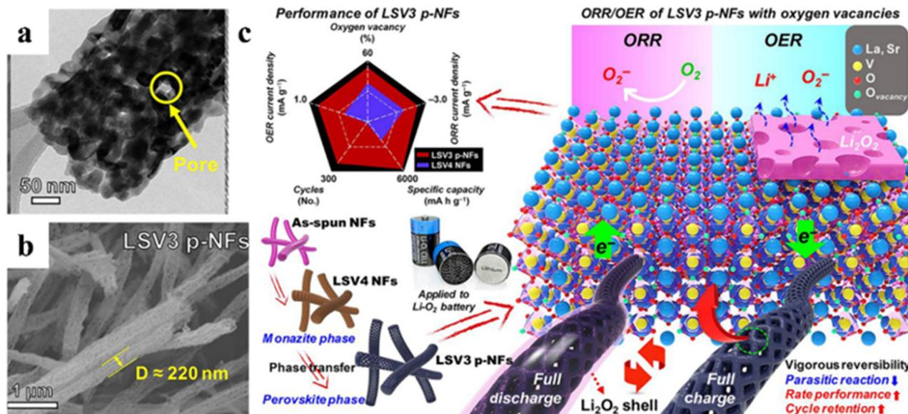
Fig. 13 TEM (a) and SEM (b) of  $\text{La}_{0.8}\text{Sr}_{0.2}\text{VO}_3$  (LSV3 p-NFs). Schematic illustration of LSV3 p-NFs used in rechargeable Li–O<sub>2</sub> batteries (c).<sup>136</sup> Copyright © 2020 Elsevier.
