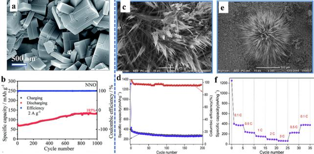
Fig. 6 SEM micrograph (a) and cycling performance (b) of NaNbO<sub>3</sub>. 81 Copyright © 2019 Royal Society of Chemistry. SEM micrographs (c and e), cycling performance (d) and rate performance (f) of nanostructured flowerlike KTaO<sub>3</sub>.82 Copyright © 2019 Elsevier.
