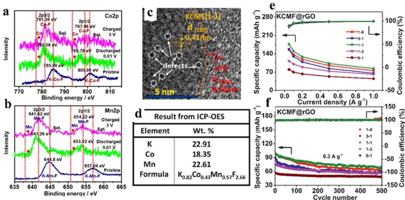
Fig. 8 Co2p (a) and Mn2p (b) of KCMF(1-1)@rGO at different voltage points (*ex situ* XPS). TEM (c) and ICP-OES (d) of KCMF(1-1)@rGO samples. The capacity and coulombic efficiency of KCMF@rGO with different Co/Mn ratios were obtained in the fifth cycle (e). Cycling stability (f).<sup>101</sup> Copyright © 2021 Elsevier.
