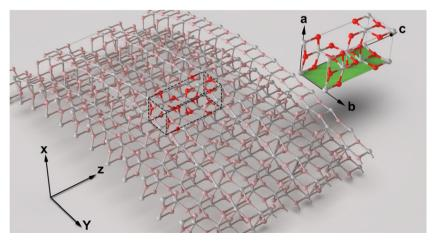
Fig. 1 The structure of the unit cell of the anatase phase of  $TiO_2$ . Only the b-c plane is assumed to interact with the ions moving through the nanotube pores.
