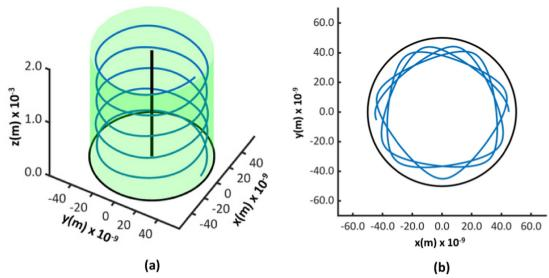
Fig. 3 Two trajectories of a single He ion (a) as seen from the side (energy:  $\sim$  2 MeV, starting position: (45, 0, 0)  $\times$  10<sup>-9</sup> m, starting velocity: (0, 7  $\times$  10<sup>-4</sup>, 1)  $\times$  9.819  $\times$  10<sup>6</sup> m s<sup>-1</sup>) (b) as seen through the cross-section (energy:  $\sim$  2 MeV, starting position: (45, 0, 0)  $\times$  10<sup>-9</sup> m, starting velocity: (0, 4  $\times$  10<sup>-4</sup>, 1)  $\times$  $9.819 \times 10^6 \ m \ s^{-1}$
