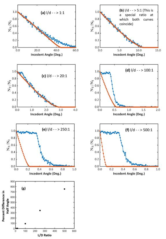
Fig. 8 (a-f) The plots show the comparison between the shadow and ion channeling effects at different nanotube aspect ratios (I/d). Both curves are normalized (brown: shadow effect, blue: channeling effect). (g) Percent difference in half angle with respect to the aspect ratio, which shows the relative effect of the channeling potential in guiding ions.  $N_T$ : # of transmitted ions,  $N_I$ : # of incident ions.
