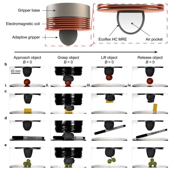
Fig. 4 Adaptive MRE gripper. (a) Schematic of an adaptive gripper consisting of an HC MRE membrane and an incorporated air pocket and test fixture. (b) Images of the adaptive gripper grasping a tomato, (c) a lego brick, (d) a marker, and (e) a cluster of grapes.
