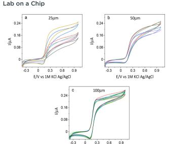
Fig. 5 Cyclic voltammograms of electrodes of different sizes (a) 25, (b) 50 and (c) 100  $\mu$ m width, 2.5 mm length in 1 mM FcDM and 0.1 M KNO $_3$  at 100 mV s $^{-1}$ . Each set of electrodes comes from the same plate.
