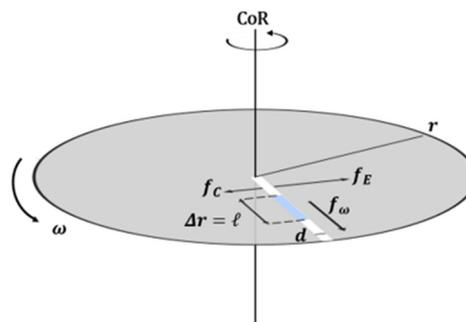
Fig. 2 Forces acting on a fluid plug propelled within a centrifugal disc. The angular frequency ( $\omega$ ) of the disc determines the magnitude of the centrifugal ( $f_\omega$ ), Coriolis ( $f_C$ ), and Euler ( $f_E$ ) forces according to opposing vectors. The liquid plug, with a diameter ( $d$ ) and absolute length ( $l = \Delta r$ ), is shown at an average radial distance ( $\bar{r}$ ) from the center of rotation (adapted from ref. 28).
