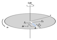
Fig. 2 Forces acting on a fluid plug propelled within a centrifugal disc. The angular frequency  $(\omega)$  of the disc determines the magnitude of the centrifugal  $(f_{\omega})$ , Coriolis  $(f_{\rm C})$ , and Euler  $(f_{\rm E})$  forces according to opposing vectors. The liquid plug, with a diameter (d) and absolute length  $(l = \Delta r)$ , is shown at an average radial distance  $(\overline{r})$  from the center of rotation (adapted from ref. 28).
