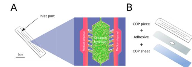
**Fig. 3** Microfluidic device appearance and components. (A) Magnified representation of a COP-MD with collagen hydrogel embedded cells (green) confined into the central chamber and culture medium perfused through the two lateral channels creating a gradient of medium. (B) Schematic illustration of the elements integrating the microfluidic device.
