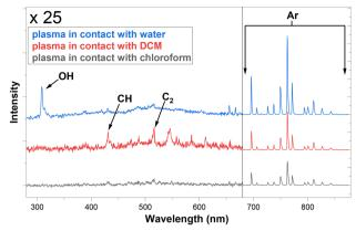
Fig. 3 OES measurements of plasma glow in contact with three solvents, recorded at the junction in the microfluidic reactors (blue
