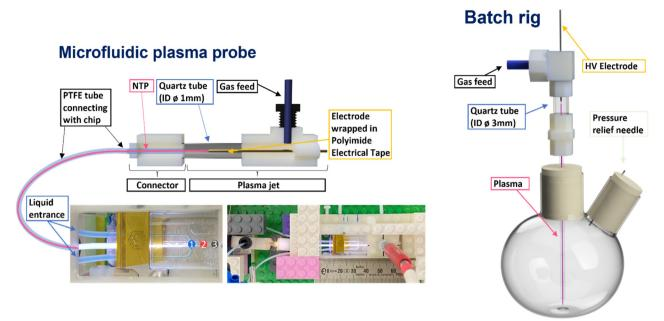
Fig. 1 Schematic representation of microfluidic and batch NTP reactors. Numbers on the microfluidic chip indicate positions where OES was performed.
