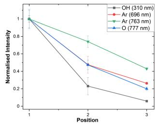
Fig. 5 Normalised peak intensities of OH, Ar, and O species observed by OES at positions 1, 2, and 3 (Fig. 1). Error bars represent by standard error taken from repeated OES measurements (n = 3).
