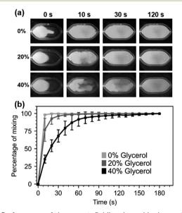
Fig. 2 Performance of the acoustofluidic mixer with viscous fluids. a) Video screenshots of 0%, 20% and 40% glycerol solutions (glycerol-DI water mixture was used in one half of the chamber, and glycerolfluorescein-tagged DI water mixture was used in the other half) at 0 s, 10 s, 30 s and 120 s time points. b) Analysis of mixing performance. Percentage of mixing was assessed by image analysis as described in materials and methods. All data acquired in triplicate.
