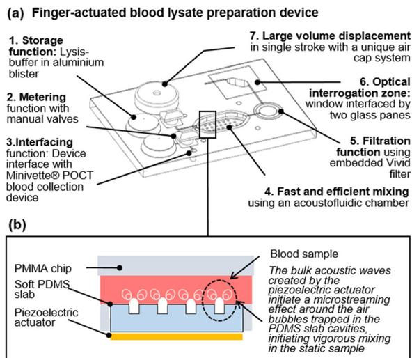
**Fig. 1** A finger-actuated filtered blood lysate preparation device. (a) Isometric CAD view of the concept, illustrating seven functional elements. (b) Illustration of the acoustic mixing principles developed in ref. 11.
