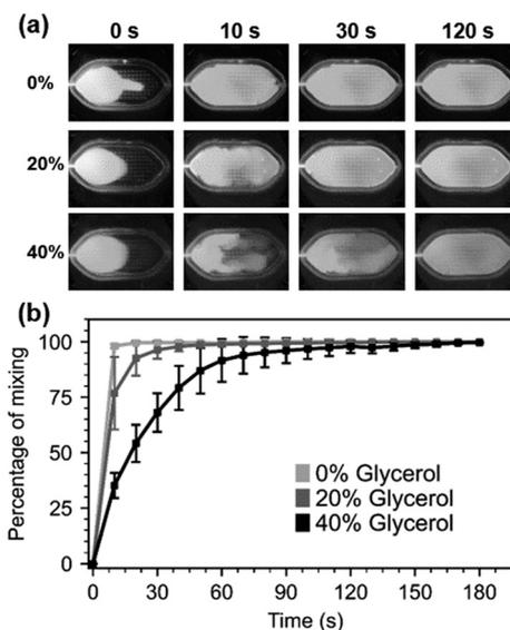
**Fig. 2** Performance of the acoustofluidic mixer with viscous fluids. a) Video screenshots of 0%, 20% and 40% glycerol solutions (glycerol–DI water mixture was used in one half of the chamber, and glycerol–fluorescein-tagged DI water mixture was used in the other half) at 0 s, 10 s, 30 s and 120 s time points. b) Analysis of mixing performance. Percentage of mixing was assessed by image analysis as described in materials and methods. All data acquired in triplicate.
