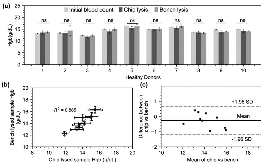
**Fig. 5** RBC lysis performed on 10 healthy donor blood samples (a) Hgb levels on ten donor samples prior to processing, and after chip and bench processing. Statistics: Anova tests within samples showed no significant difference (b) correlation between bench and chip lysates. A linear regression model was fitted with an  $R^2$  value of 0.885. (c) Bland–Altman plot showing agreement between the hemoglobin values acquired on chip and bench lysates.
