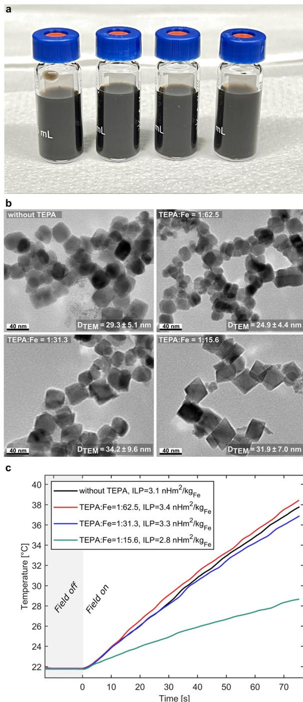
**Fig. 3** (a) IONP solutions synthesised in flow using the three-phase reactor platform. (b) TEM analysis of IONPs synthesised at different TEPA:Fe ratios. (c) Corresponding heating profiles (of washed solutions) with ILP values in the legend.
