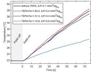
Fig. 3 (a) IONP solutions synthesised in flow using the three-phase reactor platform. (b) TEM analysis of IONPs synthesised at different TEPA: Fe ratios. (c) Corresponding heating profiles (of washed solutions) with ILP values in the legend.
