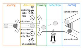
Fig. 1 The acoustic activated absorbance droplet sorter (AcAADS) can be separated into five functional regions: spacing of the droplet, absorbance detection, focusing of the droplet to the preferential flow, deflection of the droplet by SAW and sorting into the two waste outlet channel. The arrows indicate flow directions and the colour of the droplets represent different absorbance values of the droplet content.
