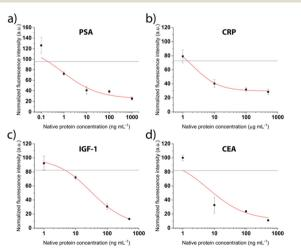
Fig. 5 Calibration curves recorded for the different targeted proteins a) PSA, b) CRP, c) IGF-1 and d) CEA. The red line corresponds to 4-parameter logistic fit and the grey line indicates background signal +  $3\times$  standard deviation for determination of the LOD (n=3).
