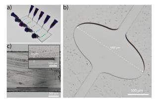
Fig. 2 a) Photograph of a sealed and connected chip incorporating five individual channels. b) Focus stack image of the imprinted channel structure into 240 µm thick COC. c) Image of the cross-section of a microfluidic channel sealed with a 2 mm thick COC slide by the solvent-assisted bonding technique (the inset shows the channel at higher resolution).
