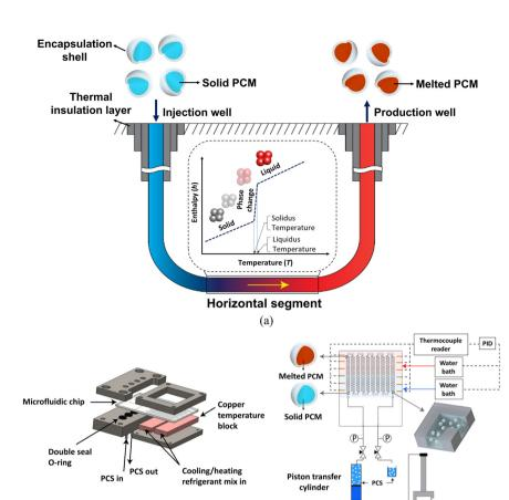
Fig. 3 Lab-on-a-chip analysis of processes relevant to geothermal energy. A closed-loop geothermal system (a) is a closed system, and can benefit from specialized working fluids. The work highlighted here employs LoC methods (b and c) to assess the potential for a microencapsulated phase change slurry as a working fluid, with testing at temperatures, pressures and shear-rates relevant to large scale operations. Reprinted with permission from ref. 121 copyright 2021 American Chemical Society.
