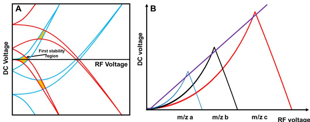
Fig. 1 (A) Shows the Mathieu stability plot for one  $m/z$ . (B) Shows the first stability region for three different  $m/z$ .
