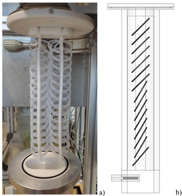
Fig. 2 Picture of the PFA digestion tube assembly retracted from the high-pressure microwave applicator (a) and side view of the computer simulation of the PFA digestion tube and the microwave antenna near the bottom of the applicator (b). Please note the different tilt angles of the PFA digestion-tube-loops in (b) that where optimized by microwave field simulation for similar power uptake for every loop.
