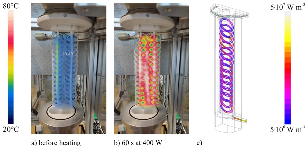
**Fig. 3** Image of the digestion coil overlaid by thermal images before (a) and after heating with 400 W for 60 s (b). The digestion coil was filled with 3% (v/v) nitric acid, though no flow was applied to identify the static heating pattern. The computer simulation of the volume loss density within the PFA digestion tube is shown in (c). Due to the symmetry of the digestion coil, only half of the microwave applicator was included in the simulation, whereby the simulation time could be reduced.
