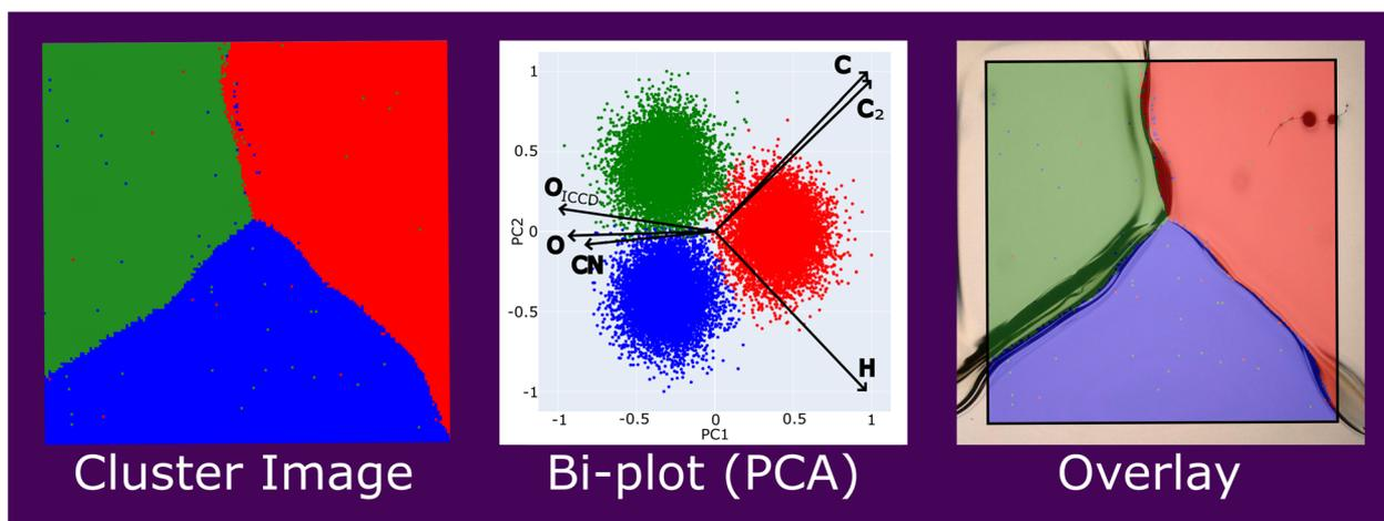
Fig. 4 Chemometric evaluation of LIBS data: cluster image (of *k*-means cluster analysis), Bi-plot of a PCA and overlay of cluster image with microscopic image. PI is depicted in green, PS in red and PVP in blue.
