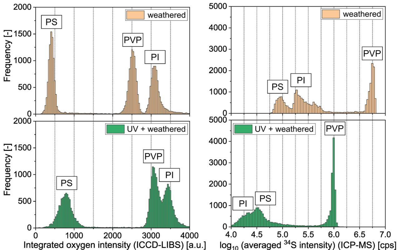
Fig. 5 Histograms for the O signal of ICCD-LIBS (bin size = 30) and  $\log_{10}({}^{34}\text{S})$  signal of LA-ICP-MS (bin size = 0.03) of images of  $\text{H}_2\text{S}$  weathered multi-polymer samples with and without prior UV treatment.
