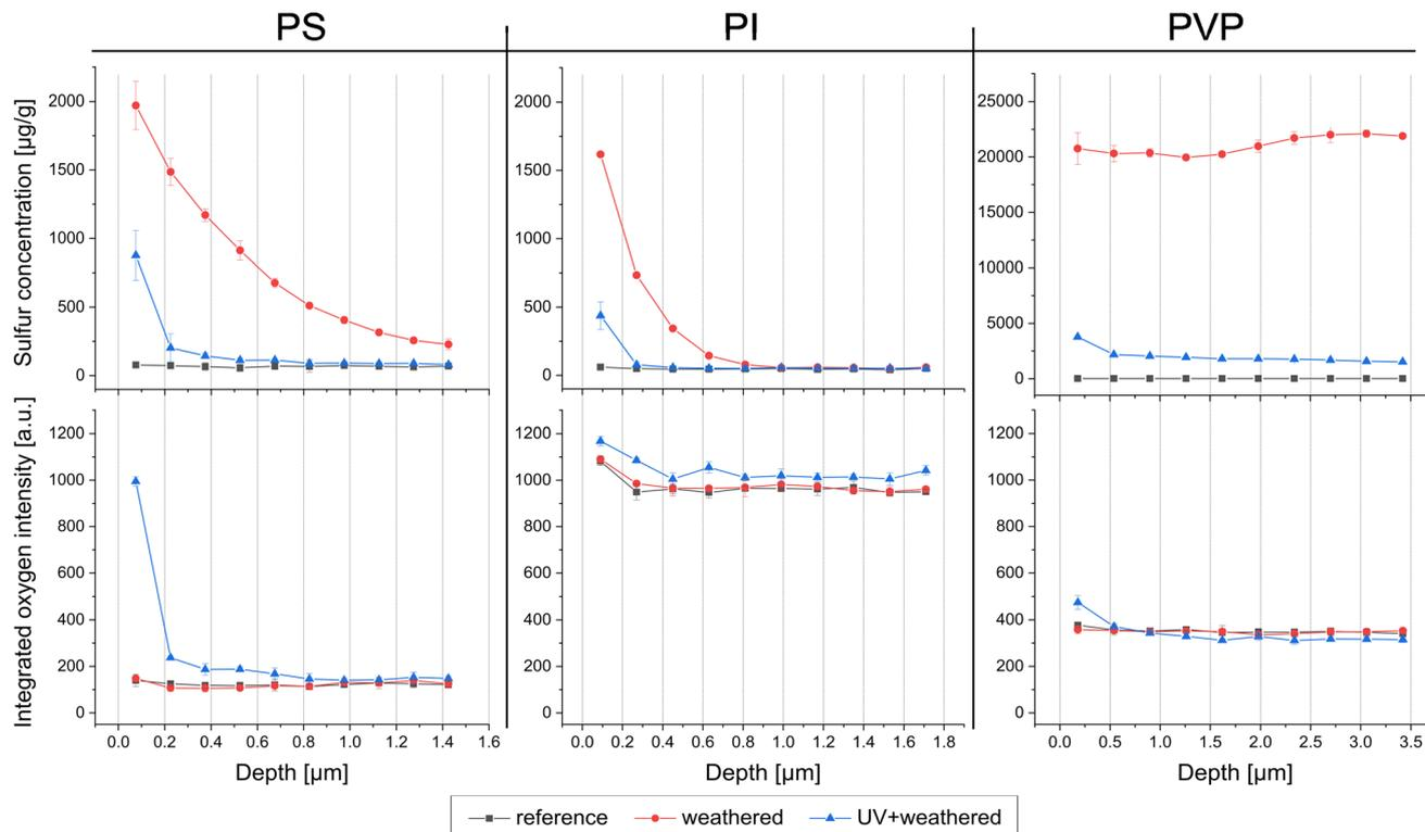
Fig. 6 Simultaneously determined quantitative sulfur depth profiles *via* LA-ICP-MS and qualitative oxygen depth profiles *via* LIBS of PS, PI, and PVP. Of each polymer type, an untreated reference, a UV-treated and subsequently weathered, and a non-UV-treated and subsequently weathered sample film was measured.
