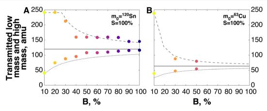
Fig. 6 Calculated low mass (dotted line) and high mass (dashed line) transmitted through the slit located between the two Wien filters as a function of the magnetic field in the first Wien filter (in %). Details for calculations are given in the ESI.† (A)  $m_0 = 120$  amu. Solid circles are from direct measurements as shown in Fig. 3 with a threshold value of 1 V. (B)  $m_0 = 63$  amu. Solid circles are from direct measurements as shown in Fig. 4 with a threshold value of 1 V.
