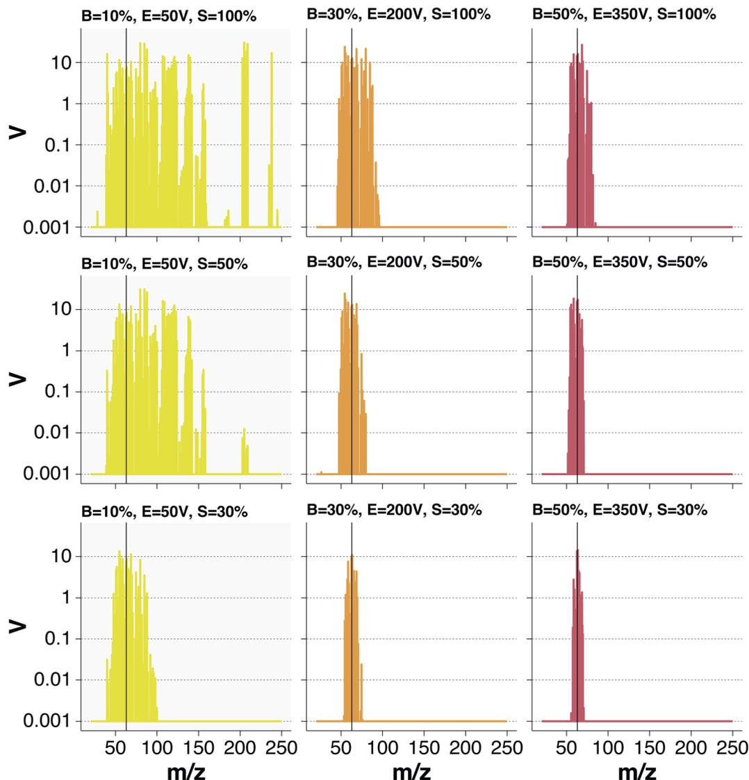
Fig. 4 Overall signal intensities for a mass scan with  $m_0 = 63$  from 20 to 250  $m/z$  for various values of induction and adjustable slit aperture. Amplifier of the axial collector was set at  $10^{11} \Omega$ .
