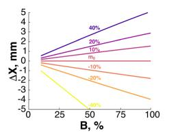
Fig. 5 Deviation in x-axis at the position of the slit located between the two Wien filters for various masses shifted by X% as labeled on the curves, as a function of magnetic field in the first Wien filter given in %. The line with no deviation corresponds to the mass  $m_0 = 120$  amu. The length of the Wien is assumed to be 7 cm and the kinetic energy of the singly charged ions is 2 keV. Details for calculations are given in the ESI.†
