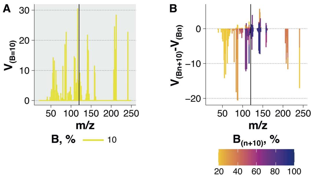
Fig. 2 A) Overall signal intensities for a mass scan with  $m_0 = 120$  from 20 to 250  $m/z$  with induction set at  $B = 10\%$ . (B) Difference of signal intensities between two successive mass scans with induction set at  $B(n + 10)$  and  $B(n)$ , with  $n$  increasing by a 10% increment. Amplifier of the axial collector was set at  $10^{11} \Omega$ .
