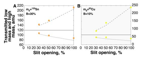
Fig. 7 Calculated low mass (dotted line) and high mass (dashed line) transmitted through the slit located between the two Wien filters as a function of the opening of the slit (in %). Details for calculations are given in the ESI.† (A)  $m_0 = 120$  amu. Solid circles are from direct measurements as shown in Fig. 3 with a threshold value of 1 V. (B)  $m_0 = 63$  amu. Solid circles are from direct measurements as shown in Fig. 4 with a threshold value of 1 V.
