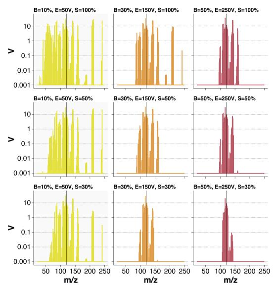
Fig. 3 Overall signal intensities for a mass scan with  $m_0 = 120$  from 20 to 250 m/z for various values of induction and adjustable slit aperture. Amplifier of the axial collector was set at  $10^{11} \Omega$ .
