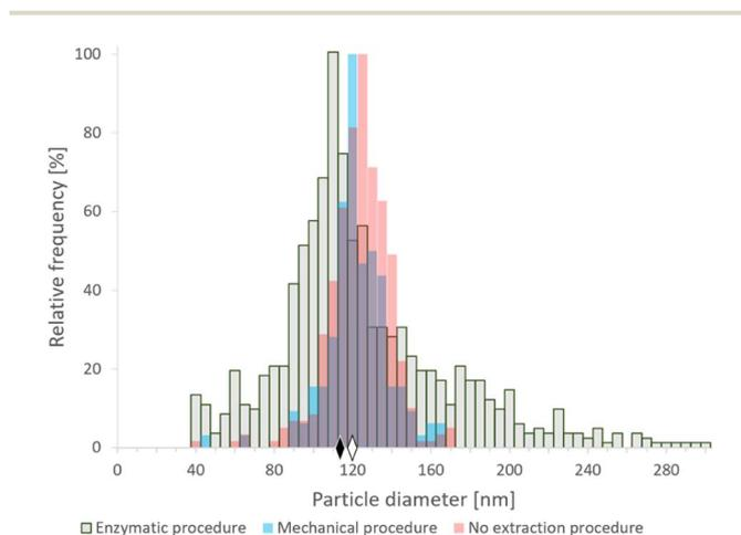
Fig. 1 SP-ICP-MS histograms of size distribution of commercial SeNPs (nominal size 150 nm) after enzymatic<sup>16</sup> (gray) and mechanical<sup>20</sup> (blue) extraction procedures, and analyzed directly after centrifugation and dilution (pink). The diamonds represent the median size of NPs after enzymatic (black) and mechanical (white) sample preparation procedures. Bin size: 5 nm.
