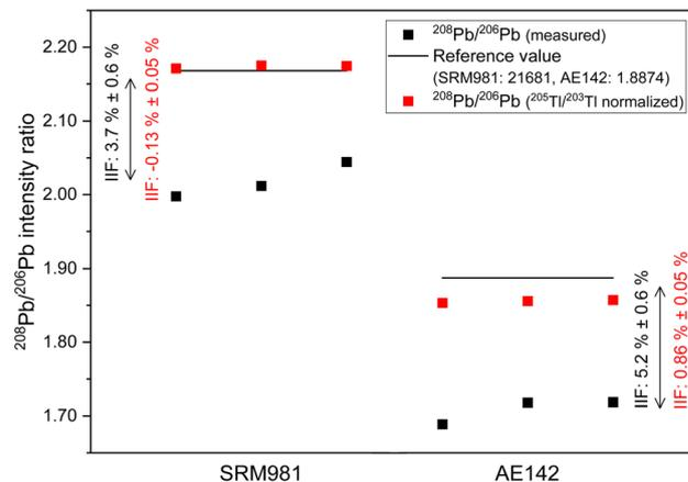
Fig. 6  $^{208}\text{Pb}/^{206}\text{Pb}$  intensity ratios and absolute  $^{208}\text{Pb}/^{206}\text{Pb}$  isotope ratios (internal inter-elemental IIF correction using Tl) for three measurements of NIST SRM 981 and ERM-AE142. Error bars (smaller than symbols) correspond to 2 s (acquisition time of 10 s,  $M = 20$ ) and are smaller than the symbols. The data shown are from the measurement of a mixture in which B, Sr, Tl and Pb were detected simultaneously.
