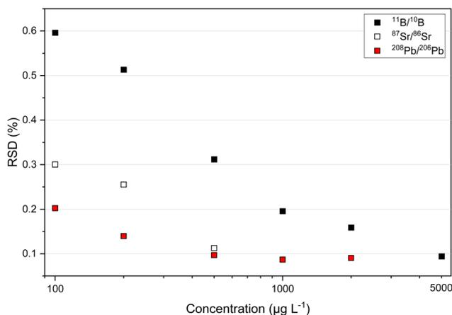
Fig. 1 Isotope ratio precision of <sup>11</sup>B/<sup>10</sup>B, <sup>87</sup>Sr/<sup>86</sup>Sr and <sup>208</sup>Pb/<sup>206</sup>Pb, expressed as RSD (%), for an acquisition time of 10 s per run ( $M$ ) and  $M = 20$ , obtained for different elemental mass concentrations. The data shown are from the measurement of a mixture in which B, Sr, and Pb were detected simultaneously.
