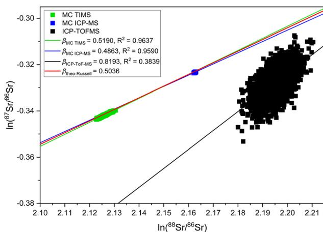
Fig. 4 Three-isotope plot for Sr from measurements over several hours of NIST SRM 987 using ICP-TOFMS (integration time 0.5 s,  $M = 2000$ ), MC TIMS (integration time 24 s,  $M = 443$ ) and MC ICP-MS (integration time 42 s,  $M = 238$ ). Solid lines represent experimentally determined slopes ( $\beta_{\text{instrument}}$ ) and predicted mass dependent fractionation line ( $\beta_{\text{theo-Russell}}$ ). All data points were taken from measurements of pure NIST SRM987 single-element solution.
