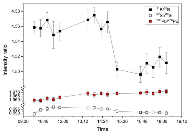
**Fig. 2** Long-term stability of  $^{11}\text{B}/^{10}\text{B}$ ,  $^{87}\text{Sr}/^{86}\text{Sr}$  and  $^{208}\text{Pb}/^{206}\text{Pb}$  isotope ratios over eight hours for 15 discontinuous measurements of NIST SRM 951a, NIST SRM 987 and NIST SRM 981. Error bars correspond to 2 s (acquisition time of 10 s,  $M = 20$ ). The data shown are from the measurement of a mixture in which B, Sr, and Pb were detected simultaneously.
