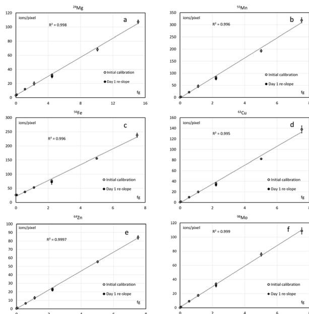
Fig. 4 Calibration curves for quantitative LA-ICP-TOFMS imaging of Mg, Mn, Fe, Cu, Zn and Mo (a–f) in tissue samples at  $3\ \mu\text{m}$  spot size. Error bars correspond to 1sd between individual cryosections ( $n = 3$ ,  $30\ \mu\text{m}$  thickness) of spiked gelatin.
