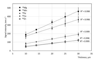
Fig. 3  $^{24}$ Mg,  $^{55}$ Mn,  $^{56}$ Fe,  $^{63}$ Cu, and  $^{64}$ Zn signal intensity as a function of gelatin cryosection thickness. Concentration of spikes is approximately 670 mg kg $^{-1}$  of dry gelatin for Mg and 330 mg kg $^{-1}$  of dry gelatin for Mn, Fe, Cu and Zn. Error bars correspond to 1sd between signals from individual sections (n=4).
