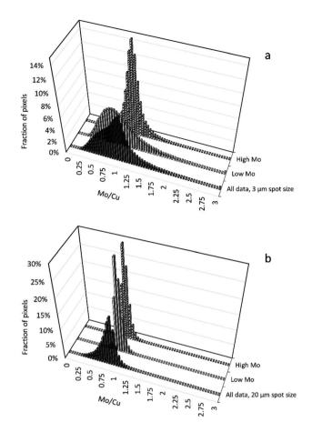
Fig. 7 Histograms of Mo/Cu ratio distribution in single pixels of a kidney section taken from a rat given 60 mg per kg per day bischoline tetrathiomolybdate (TTM) imaged at 3  $\times$  3  $\mu m$  (a) and 20  $\times$  18  $\mu m$  pixel size (b). Data for low Mo concentration (<64 mg kg $^{-1}$ ) and high Mo concentration (>64 mg kg $^{-1}$ ) are shown separately.
