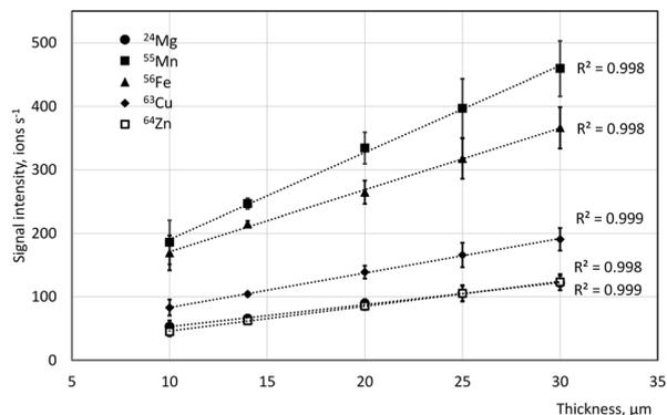
Fig. 3 <sup>24</sup>Mg, <sup>55</sup>Mn, <sup>56</sup>Fe, <sup>63</sup>Cu, and <sup>64</sup>Zn signal intensity as a function of gelatin cryosection thickness. Concentration of spikes is approximately 670 mg kg<sup>-1</sup> of dry gelatin for Mg and 330 mg kg<sup>-1</sup> of dry gelatin for Mn, Fe, Cu and Zn. Error bars correspond to 1sd between signals from individual sections ( $n = 4$ ).
