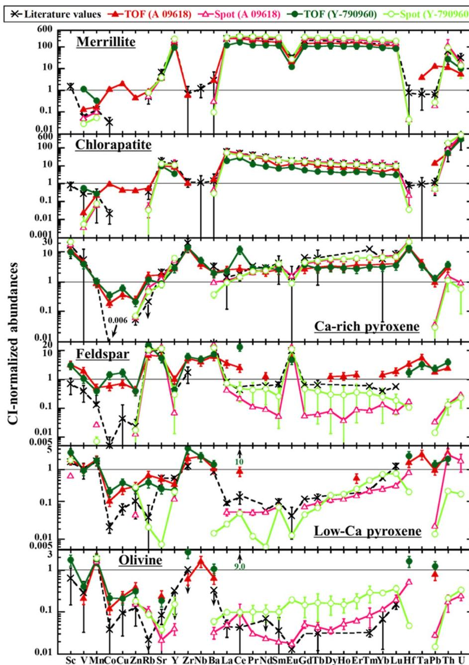
Fig. 7 CI-normalized abundances of trace elements in constituent minerals as obtained using LA-ICP-TOF-MS mapping (TOF) and LA-ICP-SF-MS spot analysis (spot) to the corresponding literature values.<sup>39,40,42,45,46</sup> See ESI Tables 4–9† for the details on the uncertainties. Error bars may be smaller than the symbol size. CI values are from Anders and Grevesse (1989).<sup>47</sup>
