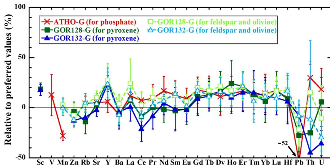
Fig. 2 Bias (%) between the elemental abundances in reference materials obtained using LA-ICP-SF-MS spot analysis and the corresponding preferred values.<sup>35</sup> The error bars represent 1 SD.
