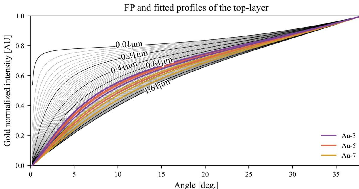
Fig. 8 (Black) FP-profiles; different colour: fitted profiles for the  $L_{\alpha}$  line of gold, each colour representing a sample. The number represents the thickness of the golden layer of the FP-calculated profiles.
