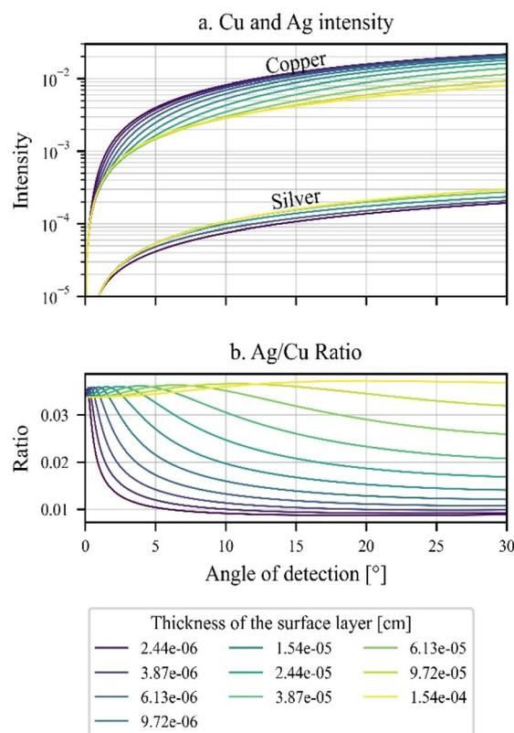
**Fig. 2** (a) Silver and copper intensities calculated for a coin sample with a bulk composition of 60% silver and a surface layer of 80% silver, the plots represent different profiles calculated for different thicknesses of the surface layer. (b) Ratio of the silver and copper intensity.
