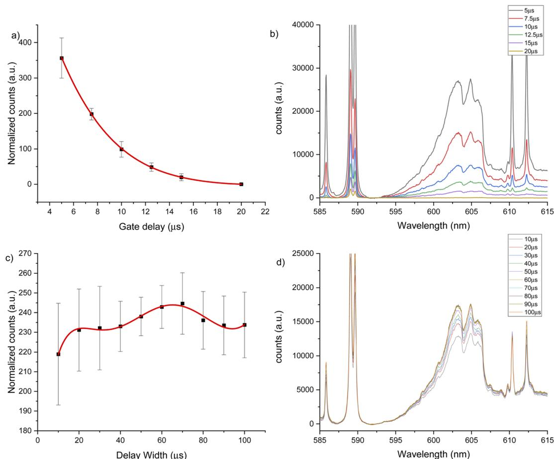
Fig. 5 LIBS signal optimization under helium flow of  $1 \text{ L min}^{-1}$  for 600 nm window using a  $2500 \mu\text{g g}^{-1}$  hydroxyapatite standard. (a) Gate delay optimization maintaining constant gate width at  $50 \mu\text{s}$ . (b) LIBS spectrum for each gate delay change, (c) gate width optimization maintaining constant gate delay at  $10 \mu\text{s}$ . (d) LIBS spectrum for each gate width change.
