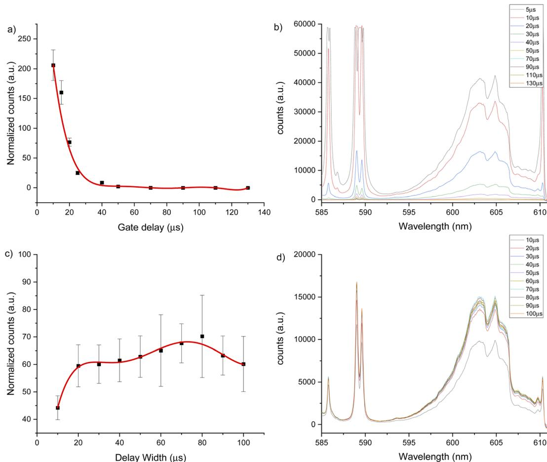
Fig. 4 LIBS signal optimization under argon flow of 1 L min<sup>-1</sup> for 600 nm window using a 2500 μg g<sup>-1</sup> hydroxyapatite standard. (a) Gate delay optimization maintaining constant gate width at 50 μs, (b) LIBS spectrum for each gate delay change, (c) gate width optimization maintaining constant gate delay at 20 μs, (d) LIBS spectrum for each gate width change.
