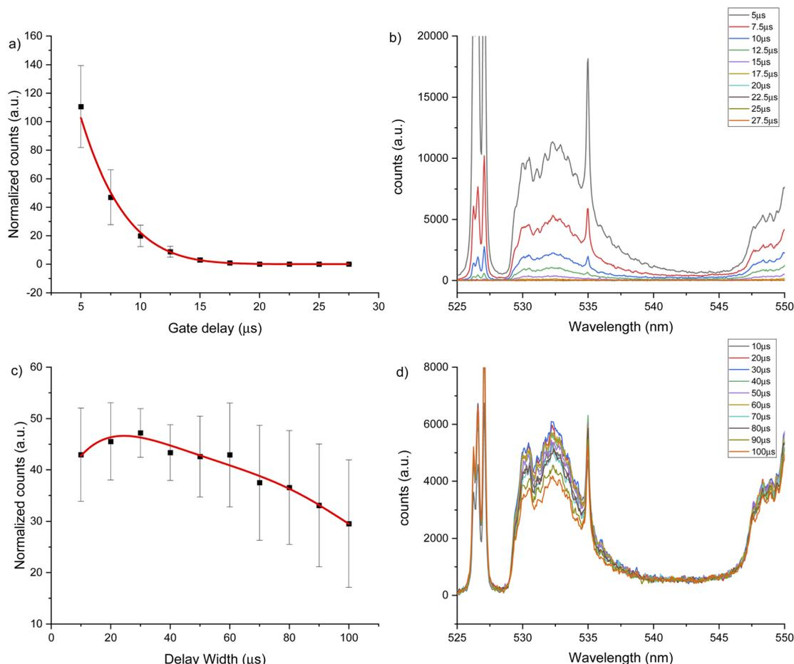
Fig. 3 LIBS signal optimization under helium flow of  $1 \text{ L min}^{-1}$  for 530 nm window using a  $2500 \mu\text{g g}^{-1}$  hydroxyapatite standard. (a) Gate delay optimization maintaining constant gate width at  $50 \mu\text{s}$ , (b) LIBS spectrum for each gate delay change, (c) gate width optimization maintaining constant gate delay at  $10 \mu\text{s}$ , (d) LIBS spectrum for each gate width change.
