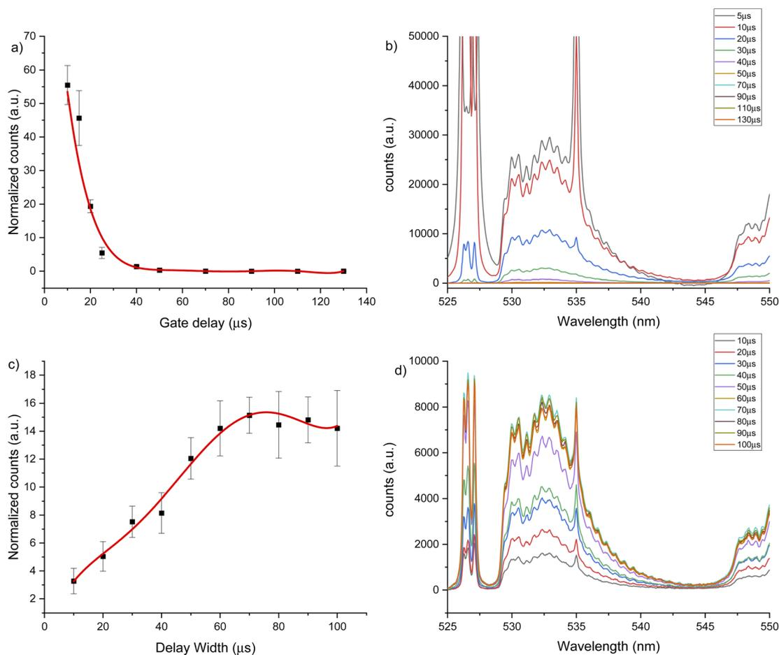
Fig. 2 LIBS signal optimization under argon flow of  $1 \text{ L min}^{-1}$  for  $530 \text{ nm}$  window using a  $2500 \mu\text{g g}^{-1}$  hydroxyapatite standard. (a) Gate delay optimization maintaining constant gate width at  $50 \mu\text{s}$ , (b) LIBS spectrum for each gate delay change, (c) gate width optimization maintaining constant gate delay at  $20 \mu\text{s}$ , (d) LIBS spectrum for each gate width change.
