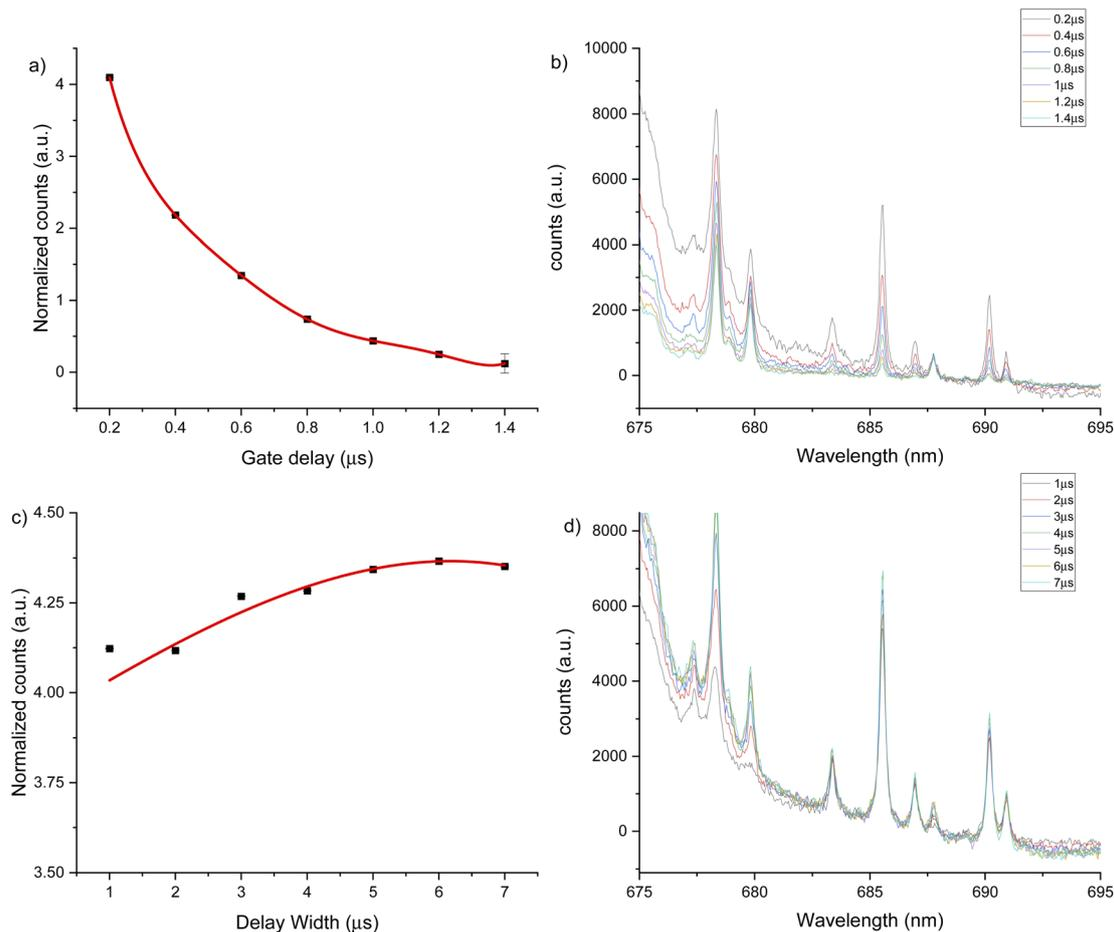
Fig. 6 LIBS signal optimization under helium flow of  $1 \text{ L min}^{-1}$  for 689 nm window using a  $2500 \mu\text{g g}^{-1}$  hydroxyapatite standard. (a) Gate delay optimization maintaining constant gate width at  $4 \mu\text{s}$ , (b) LIBS spectrum for each gate delay change, (c) gate width optimization maintaining constant gate delay at  $0.2 \mu\text{s}$ , (d) LIBS spectrum for each gate width change. Error bars on (a) and (c) are too small to be seen.
