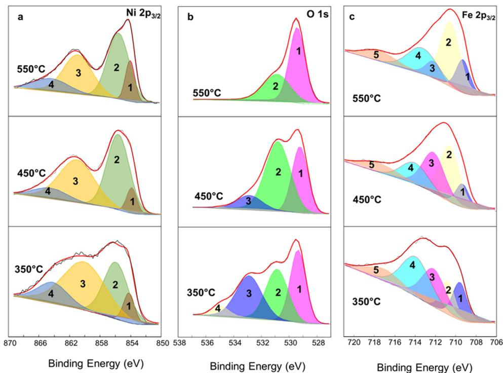
Fig. 4 Comparison of XPS deconvolution for (a) Ni 2p<sub>3/2</sub>; (b) O 1s and (c) Fe 2p<sub>3/2</sub> signals.
