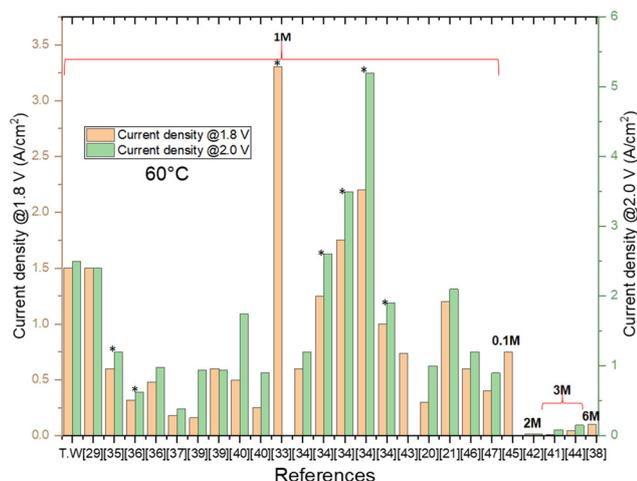
Fig. 7 Comparison at 60 °C among the values of current densities from the literature obtained at 1.8 V and 2.0 V, with different KOH concentrations. \* corresponds to cells based on noble metals at both anode and cathode.
