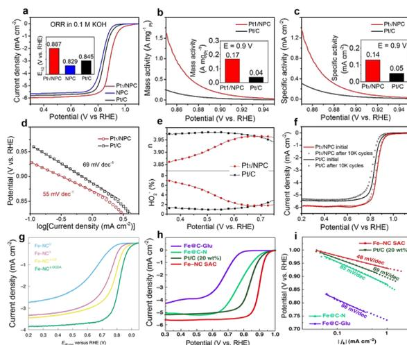
**Fig. 3** (a–f) The ORR performance of single-atom platinum catalysts. Reprinted with permission from ref. 77. Copyright 2021, Elsevier; (g) The ORR activity of a single-atom Fe catalyst. Reprinted with permission from ref. 44. Copyright 2022, Springer Nature; (h and i) Steady-state ORR polarization curves and corresponding Tafel of Fe-NC SAC, Pt/C and control samples. Reprinted with permission from ref. 38. Copyright 2019, Springer Nature.
