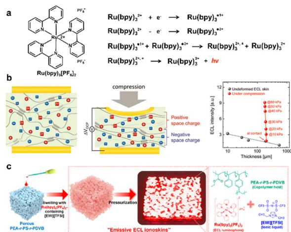
Fig. 11 (a) The reaction process of the ionic electrochemical luminescence reaction. (b) The redistribution of luminescent ions and the change in the corresponding light intensity induced by the piezoelectric effect. Reproduced with permission from ref. 25, copyright 2021, Wiley-VCH; (c) pressure visualization of porous ionic skin based on the electrochemical luminescence mentioned in Fig. 11a. Reproduced with permission from ref. 63, copyright 2021, American Chemical Society.
