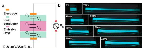
Fig. 10 (a) Schematic diagram of an electroluminescent device with ionic conductors. (b) The luminescence states of electroluminescent devices under different strains. Reproduced with permission from ref. 57, copyright 2016, Wiley-VCH.
