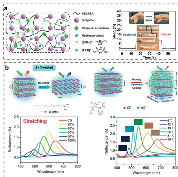
**Fig. 8** (a) Photonic ionic skin embedded with silica microspheres, and the electrical/optical responsive behavior. Reproduced with permission from ref. 49, copyright 2021, Wiley-VCH. (b) Photonic hydrogel structure based on a two-dimensional bilayer membrane and the mechanisms of optical changes by external stimulation. Reproduced with permission from ref. 47, copyright 2021, American Chemical Society.
