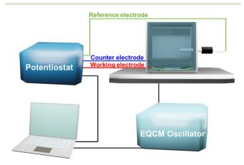
Fig. 2 Scheme of EQCM system.
