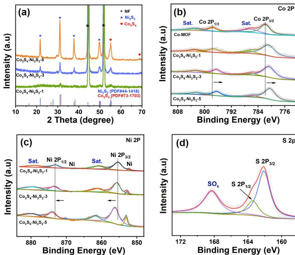
Fig. 3 (a) XRD patterns of the as-prepared  $\text{Co}_3\text{S}_4/\text{Ni}_3\text{S}_2-t$  materials at different sulfurization times ( $t = 1$  h, 3 h, and 5 h). (b) Co 2p XPS region, (c) Ni 2p XPS region and (d) S 2p XPS region.
