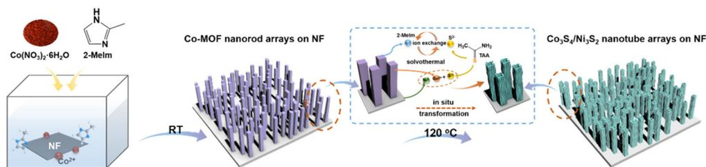
**Fig. 1** Transformation of Co-MOF nanorod arrays on nickel foam into  $\text{Co}_3\text{S}_4$ - $\text{Ni}_3\text{S}_2$  nanotube arrays using ethanol with thioacetamide (TAA) under solvothermal conditions showing  $\text{Ni}^{2+}$  exfoliation, ion-ion reaction, ionic exchange and doping mechanisms that cause simultaneous Co-MOF nanorod decay and  $\text{Co}_3\text{S}_4$ - $\text{Ni}_3\text{S}_2$  nanotube growth.
