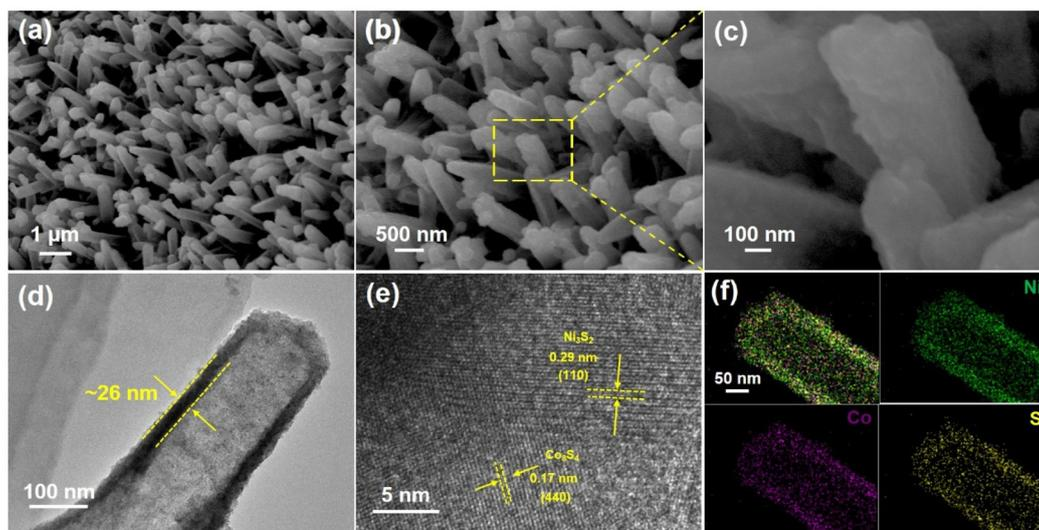
**Fig. 2**  $\text{Co}_3\text{S}_4/\text{Ni}_3\text{S}_2$ -3 nanotube arrays obtained after solvothermal sulfurization: (a–c) SEM images with different magnifications, (d) TEM image, (e) HRTEM image and (f) TEM-EDS elemental mappings.
