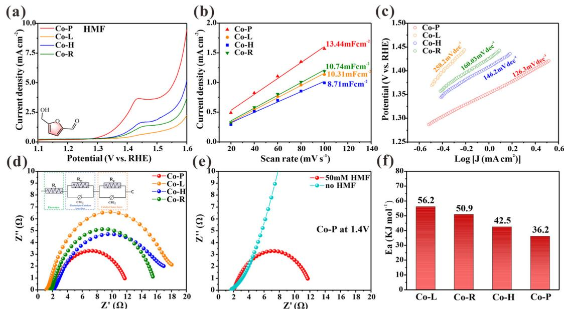
**Fig. 2** (a) LSV curves of Co-R, Co-L, Co-H and Co-P. (b) Charging current differences ( $\Delta j = j_{\text{anode}} - j_{\text{cathode}}$ ) plotted against scan rates for Co-R, Co-L, Co-H and Co-P. (c) Tafel slopes derived from LSVs. (d) Nyquist plots for Co-R, Co-L, Co-H and Co-P in 1.0 M KOH with 50 mM HMF at 1.4 V vs. RHE. (e) Nyquist plots for Co-P in 1.0 M KOH with and without 50 mM HMF at 1.4 V vs. RHE. (f) The average activation energy of Co-R, Co-L, Co-H and Co-P.
