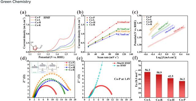
Fig. 2 (a) LSV curves of Co-R, Co-L, Co-H and Co-P. (b) Charging current differences ( $\Delta j = j_{\rm anode} - j_{\rm cathode}$ ) plotted against scan rates for Co-R, Co-L, Co-H and Co-P. (c) Tafel slopes derived from LSVs. (d) Nyquist plots for Co-R, Co-L, Co-H and Co-P in 1.0 M KOH with 50 mM HMF at 1.4 V vs. RHE. (e) Nyquist plots for Co-P in 1.0 M KOH with and without 50 mM HMF at 1.4 V vs. RHE. (f) The average activation energy of Co-R, Co-L, Co-H and Co-P.
