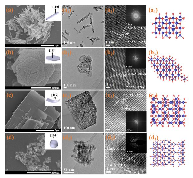
Fig. 1 SEM and TEM images of Co-R (a and a<sub>1</sub>), Co-H (b and b1), Co-L (c and c<sub>1</sub>) and Co-P (d and d<sub>1</sub>) (insets show the corresponding 3D models of Co<sub>3</sub>O<sub>4</sub>), a<sub>2</sub>, b<sub>2</sub>, c<sub>2</sub> and d<sub>2</sub> show the corresponding high-resolution images and SAED patterns. Surface atomic structure models of (110), (111), (112) and (114) facets ( $a_3$ ,  $b_3$ ,  $c_3$  and  $d_3$ ).
