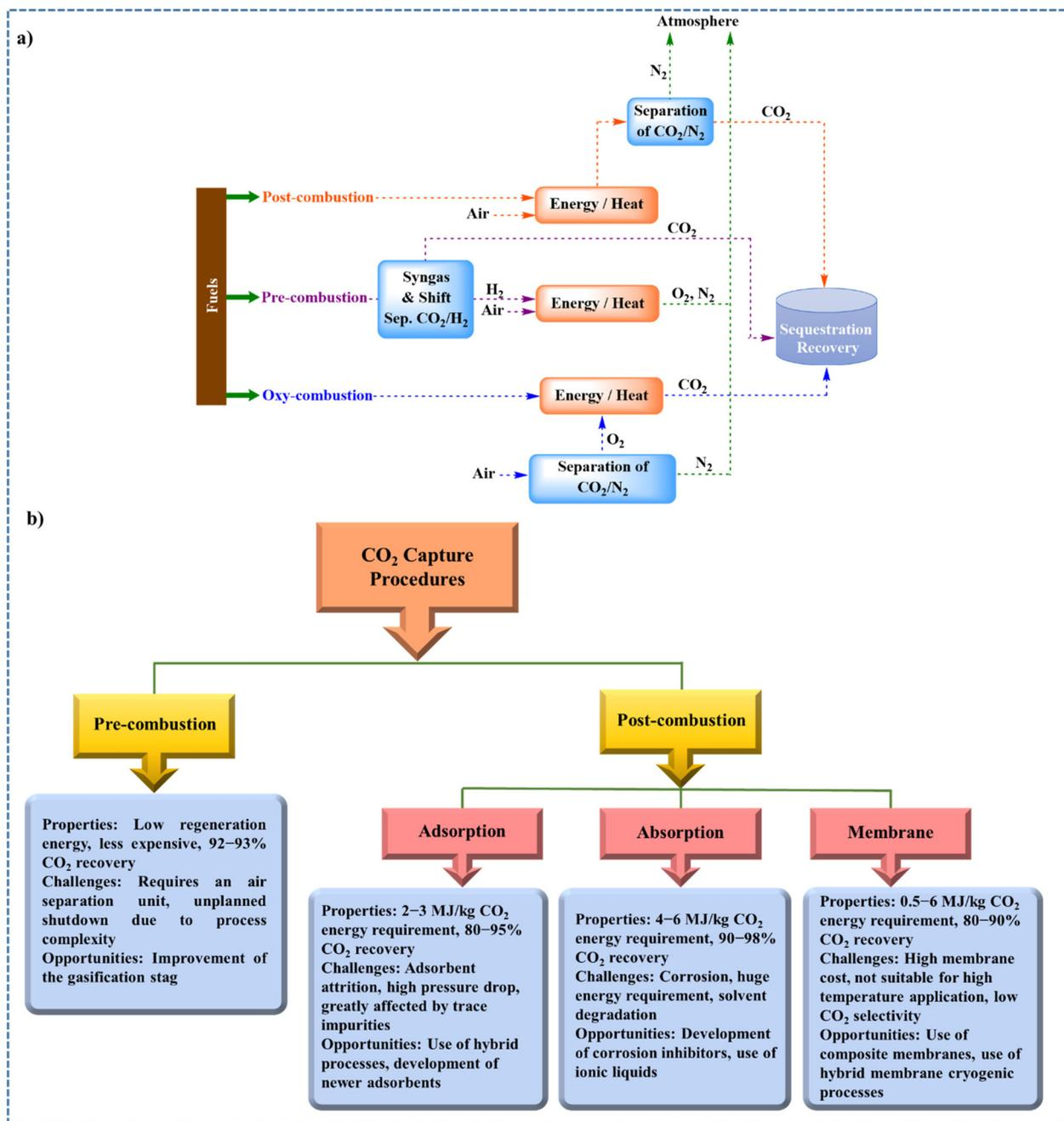
Fig. 2 Schematic representation of (a) CO<sub>2</sub> capture processes by post-, pre-, and oxy-combustion and (b) different properties of the two methods for CO<sub>2</sub> capture.<sup>13</sup>
