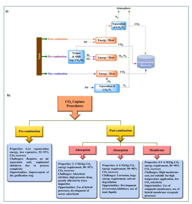
Fig. 2 Schematic representation of (a) CO<sub>2</sub> capture processes by post-, pre-, and oxy-combustion and (b) different properties of the two methods for CO<sub>2</sub> capture. 13
