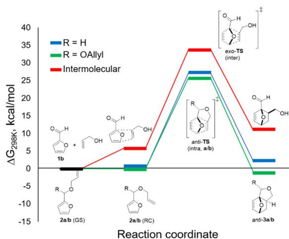
**Fig. 3** DFT mechanism (calculated with B3LYP at 6-311+g(d) and GD3BJ dispersion, in methanol (SMD)); only the paths leading to the *anti*-**3** adducts were calculated; blue = furfuryl allyl ether **2a**; green: furfural diallyl acetal **2b**; red: intermolecular reaction between furfural and allyl alcohol; GS = ground state, RC = reactive conformation.
