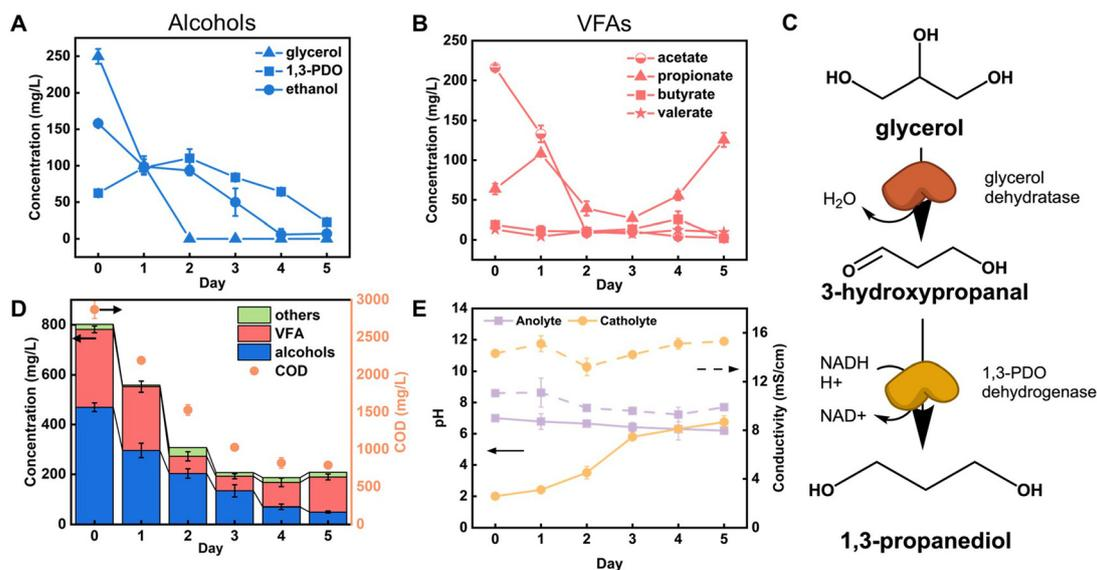
**Fig. 2** The concentration profile of (A) alcohols and (B) VFAs throughout the MEC treatment as identified by HPLC with an ion-exclusion column. (C) The metabolic pathway of glycerol fermentation to 1,3-PDO. (D) The combined concentration profile of HPLC identified chemicals and the COD degradation profile. (E) The pH and conductivity change of electrolyte throughout the MEC treatment. pH is presented by solid lines and conductivity by dashed line.
