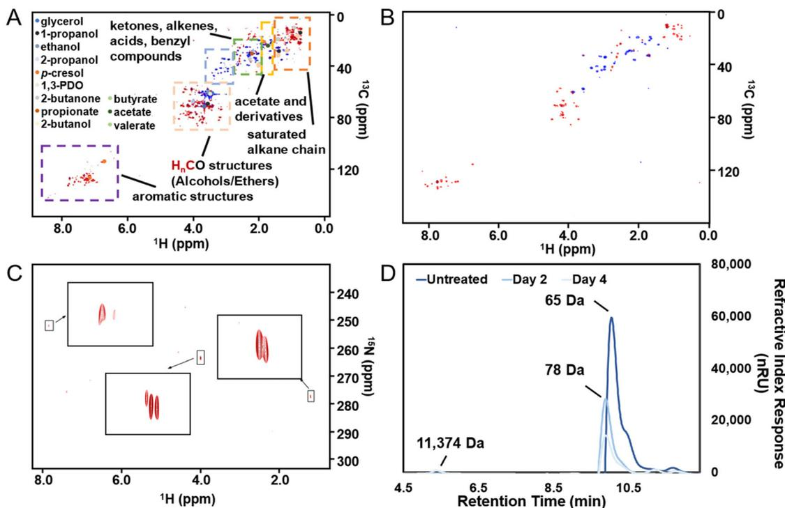
**Fig. 3**  $^1\text{H}$ - $^{13}\text{C}$  HSQC NMR spectra of (A) untreated PHW; (B) PHW after 5 days of MEC treatment. Note that the edited HSQC shows  $\text{CH}_2$  in blue and  $\text{CH}/\text{CH}_3$  in red. (C)  $^1\text{H}$ - $^{15}\text{N}$  HMBC NMR spectrum of untreated PHW, with the insets showing enlarged view of each peak. (D) Size-exclusion chromatography of PHW at different stages of MEC treatment.
