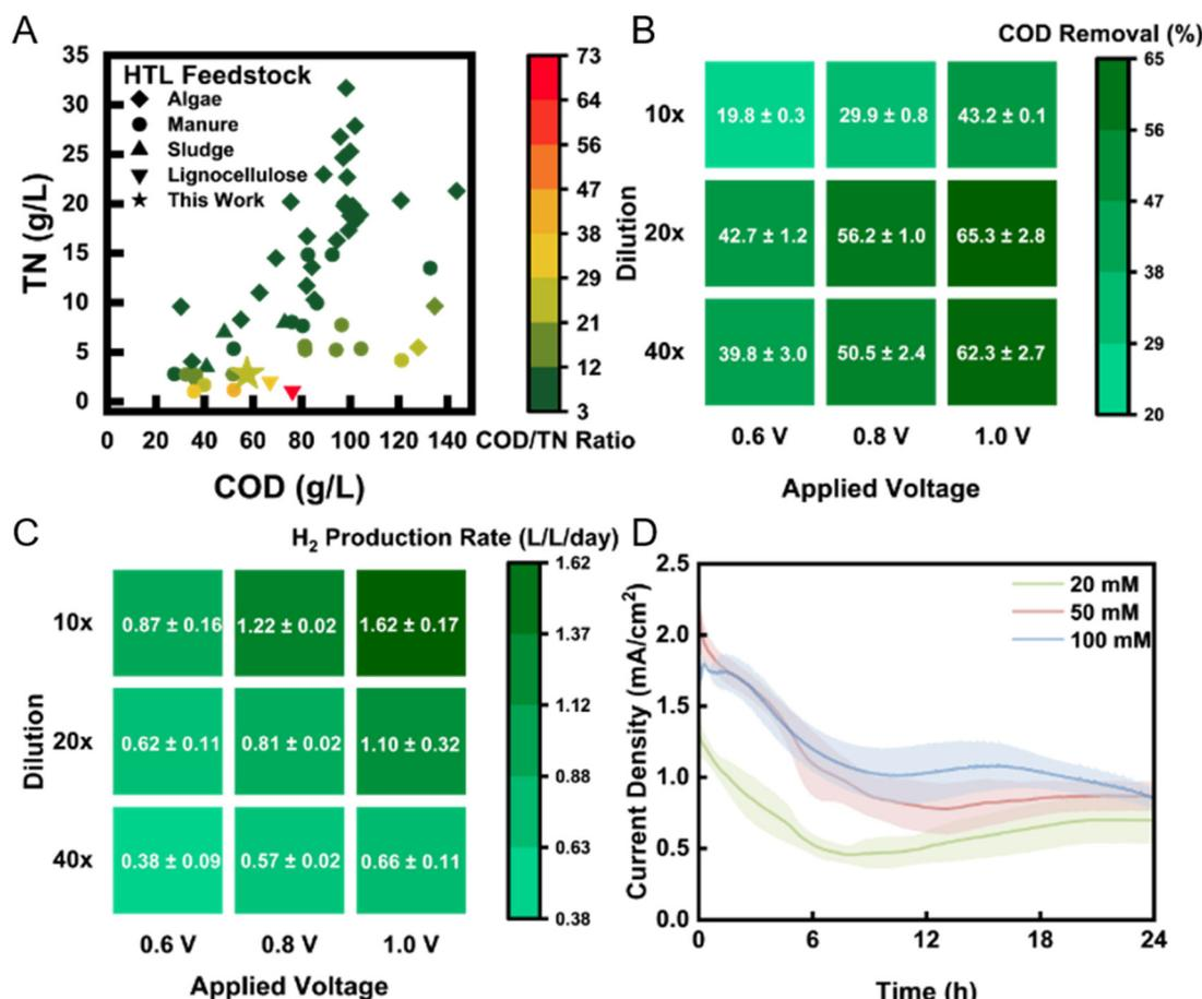
**Fig. 1** (A) COD/TN composition of feedstock PHW used in this study and other PHW studies. Literature data were collected from Watson *et al.* (2020).<sup>27</sup> The COD removal (B) and  $\text{H}_2$  production rate (C) of PHW-fed MEC in 3-day period under different applied voltage and dilution ratio. (D) The current density profile under different buffer strength after introduction of fresh electrolyte. The shadows represent standard deviation from triplicate experiments.
