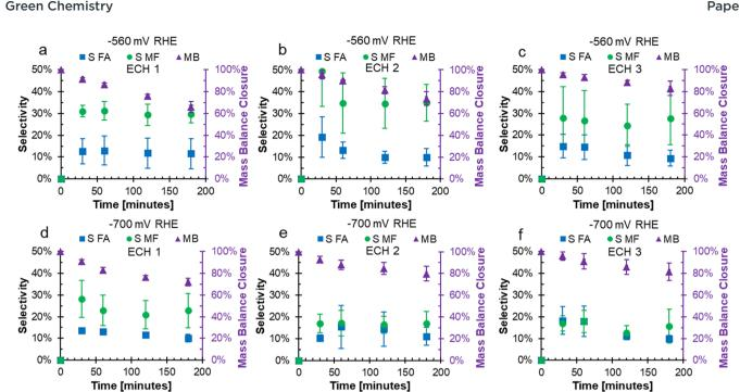
Fig. 2 Mass balance and selectivity to FA and MF from consecutive ECH of FF with recycled Cu foil electrode. At -560 mV RHE: (a) ECH1, (b) ECH2, (c) ECH3. At -700 mV RHE: (d) ECH1, (e) ECH2, (f) ECH3. Conditions: 200 mM FF, 0.5 M H<sub>2</sub>SO<sub>4</sub>, 80: 20 vol% water: acetonitrile, 3 hours duration ECH, 60 mL N<sub>2</sub> sparging, Cu electrode.
