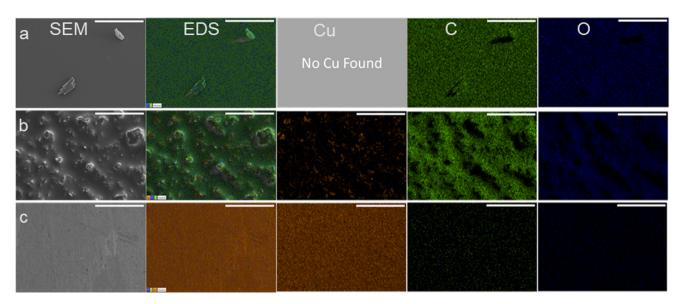
Fig. 3 SEM/EDX images at 500x magnification for (a) -560 mV RHE fouled Cu (used three times), (b) -700 mV RHE fouled Cu (used three times), (c) bare Cu. Scale bar shown is 100 µm for all images. Columns from left to right are labeled on top row.
