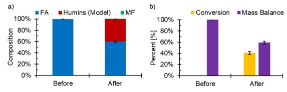
Fig. 8 (a) The composition of the FA ECH electrolyte before and after 3 h ECH. (b) The conversion and mass balance from FA ECH experiments. Conditions: -560 mV RHE, 80: 20 vol% acetonitrile: water, 0.5 M H<sub>2</sub>SO<sub>4</sub>, 15 mM FA, N<sub>2</sub> sparging 60 mL min<sup>-1</sup>, Cu electrode.
