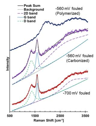
**Fig. 6** Raman spectra of -700 mV RHE fouled Cu showing D, G, and 2D bands, spectra of -560 mV RHE fouled Cu showing spectra from a carbonized area of electrode and a polymerized area of the electrode.
