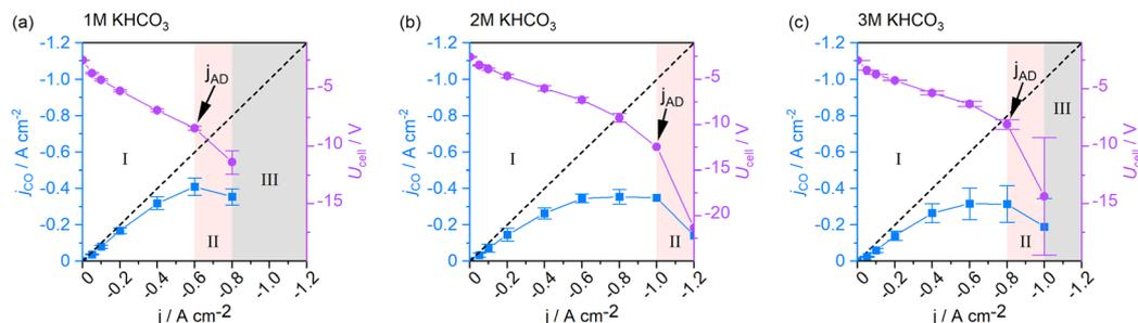
**Fig. 7** Cell voltage and CO-specific current density throughout GDE screenings using (a) 1 M, (b) 2 M, and (c) 3 M electrolytes. Regime I: steady-state cell operation, regime II: cell operation with accelerated GDE degradation, regime III: inaccessible region.
