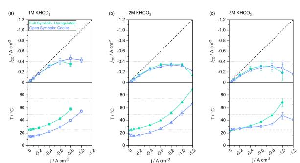
Fig. 6 CO-specific current densities and temperature evolution throughout the chrono-potentiometric screenings at varied electrolyte concentrations with vs without electrolyte cooling. (a) 1 M electrolytes, (b) 2 M electrolytes, and (c) 3 M electrolytes.
