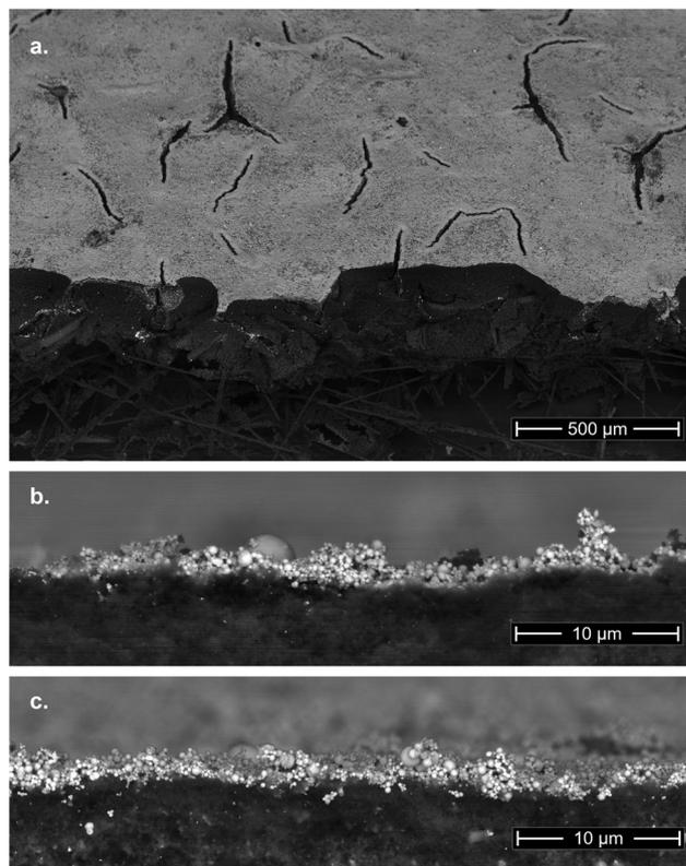
**Fig. 3** SEM micrographs of Ag-coated electrodes (a and b) before and (c) after electrolysis. (a) 45° top view of the catalyst layer on the electrode surface (BSE-detector). (b) Catalyst layer cross-section of the GDE before electrolysis (BSE-detector). (c) Catalyst layer cross-section of the GDE after electrolysis (BSE-detector).
