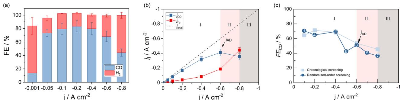
**Fig. 2** GDE performance measured in terms of (a) the CO-Faraday efficiency, (b) the product-specific current density, and  $j_{AD}$  (indication arrow). Randomized-order screenings confirmed the representativity of the data (c).
