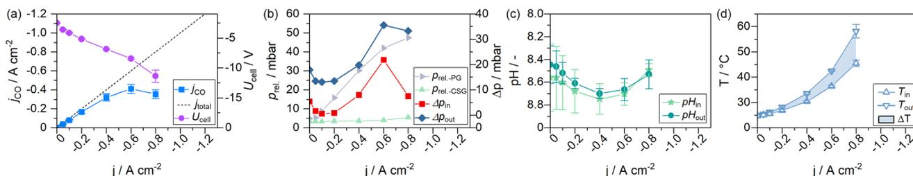
**Fig. 4** Current-dependent steady-states of a GDE flow cell operated with 1 M electrolytes. (a) Voltage and CO-specific current density, (b) relative system pressures (PG – product gas, CSG – catholyte sweep gas), (c) and the catholyte pH entering and exiting the GDE flow cell, and (d) the catholyte temperatures entering and exiting the flow cell.
