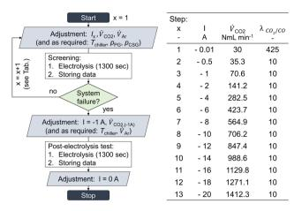
Fig. 1 Electrochemical GDE testing parameters and procedure. Chrono-potentiometric screening continued until either GDE flooding occurred or cell voltage peaks exceeded the potentiostat's compliance voltage ( $\pm 20$  V).
