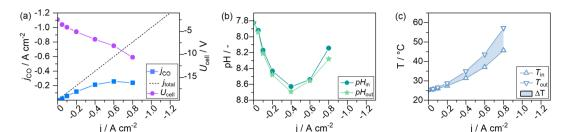
Fig. 9 Current-dependent steady-states of a GDE flow cell operated at a constant  $CO_2$  feed rate ( $\dot{V}_{CO_2} = 282.5 \, \text{mL}_n \, \text{min}^{-1}$ ). (a) Cell voltage and CO-specific current density, (b) catholyte pH entering and exiting the GDE flow cell, and (c) catholyte temperatures entering and exiting the flow cell.
