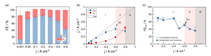
Fig. 2 GDE performance measured in terms of (a) the CO-Faraday efficiency, (b) the product-specific current density, and  $j_{AD}$  (indication arrow). Randomized-order screenings confirmed the representativity of the data (c).
