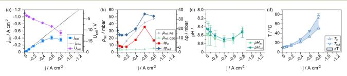
Fig. 4 Current-dependent steady-states of a GDE flow cell operated with 1 M electrolytes. (a) Voltage and CO-specific current density, (b) relative system pressures (PG - product gas, CSG - catholyte sweep gas), (c) and the catholyte pH entering and exiting the GDE flow cell, and (d) the catholyte temperatures entering and exiting the flow cell.
