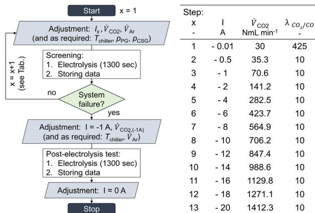
**Fig. 1** Electrochemical GDE testing parameters and procedure. Chrono-potentiometric screening continued until either GDE flooding occurred or cell voltage peaks exceeded the potentiostat's compliance voltage ( $\pm 20$  V).
