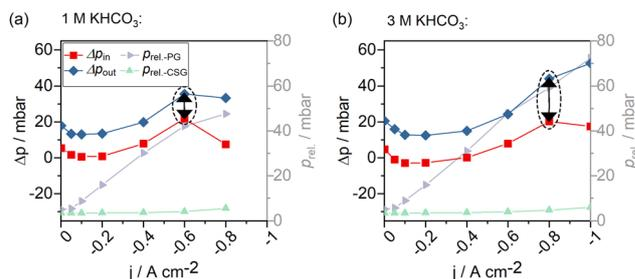
**Fig. 10** Pressure evolution in a GDE flow cell operated with (a) 1 M electrolytes and (b) 3 M electrolytes.  $\Delta p_{\text{in}}$ : Differential liquid-to-gas pressure at the GDE – cell entry,  $\Delta p_{\text{out}}$ : differential liquid-to-gas pressure at the GDE – cell exit,  $p_{\text{rel.-PG}}$ : relative pressure in the product gas stream,  $p_{\text{rel.-CSG}}$ : relative pressure in the catholyte sweep gas stream.
