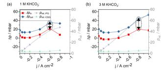
Fig. 10 Pressure evolution in a GDE flow cell operated with (a) 1 M electrolytes and (b) 3 M electrolytes.  $\Delta p_{\rm in}$ : Differential liquid-to-gas pressure at the GDE – cell entry,  $\Delta p_{\rm in}$ : differential liquid-to-gas pressure at the GDE – cell exit,  $p_{\rm rel-PG}$ : relative pressure in the product gas stream,  $p_{\rm rel-CSG}$ : relative pressure in the catholyte sweep gas stream.
