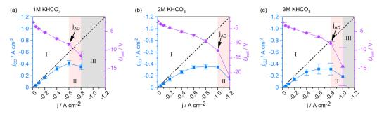
Fig. 7 Cell voltage and CO-specific current density throughout GDE screenings using (a) 1 M, (b) 2 M, and (c) 3 M electrolytes. Regime I: steady-state cell operation, regime II: cell operation with accelerated GDE degradation, regime III: inaccessible region.
