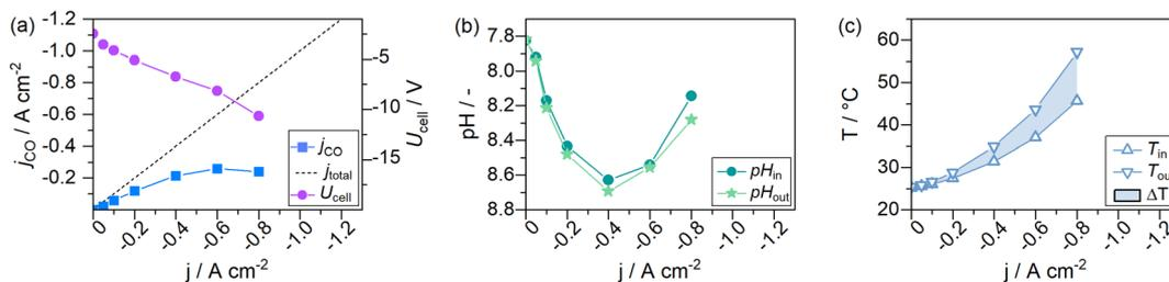
**Fig. 9** Current-dependent steady-states of a GDE flow cell operated at a constant CO<sub>2</sub> feed rate ( $\dot{V}_{\text{CO}_2} = 282.5 \text{ mL}_n \text{ min}^{-1}$ ). (a) Cell voltage and CO-specific current density, (b) catholyte pH entering and exiting the GDE flow cell, and (c) catholyte temperatures entering and exiting the flow cell.
