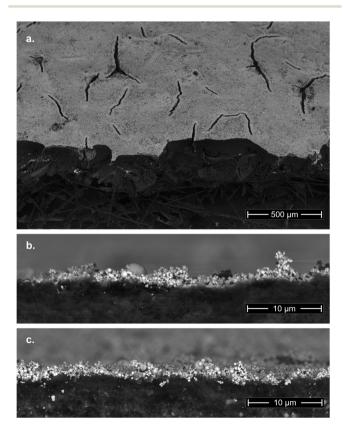
Fig. 3 SEM micrographs of Ag-coated electrodes (a and b) before and (c) after electrolysis. (a) 45° top view of the catalyst layer on the electrode surface (BSE-detector). (b) Catalyst layer cross-section of the GDE before electrolysis (BSE-detector). (c) Catalyst layer cross-section of the GDE after electrolysis (BSE-detector).
