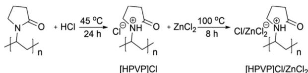
Fig. 19 Scheme of synthesis of Brønsted-Lewis [HPVP]Cl/ZnCl<sub>2</sub> deep eutectic solvent polymer via quaternization of PVP. Reproduced from ref. 65 with permission from Elsevier, 2023.
