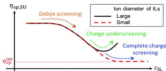
**Fig. 20** The dependence of the specific viscosity (on the Y axis) against ion concentration of IL or PIL (on the X axis) obtained from the resulting equation in ref. 71. Reproduced from ref. 71 with permission from The Royal Society of Chemistry, 2022.
