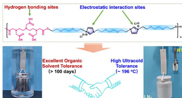
**Fig. 22** The interfacial adhesion to a combination of electrostatic interactions and hydrogen bonds, obtained from Deng *et al.*<sup>75</sup> Reproduced from ref. 75 with permission from ACS, 2022.
