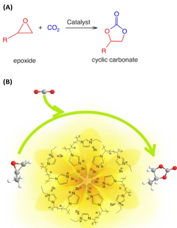
**Fig. 7** (A) Synthesis of cyclic carbonates from CO<sub>2</sub> and epoxides. Reproduced from ref. 19 with permission from CSIRO Publisher, 2021. (B) Schematic representation of CO<sub>2</sub> capture with the participation of poly(ionic liquid)s with high ionic density (HDPILs). Reproduced from ref. 20 with permission from Wiley, 2023.
