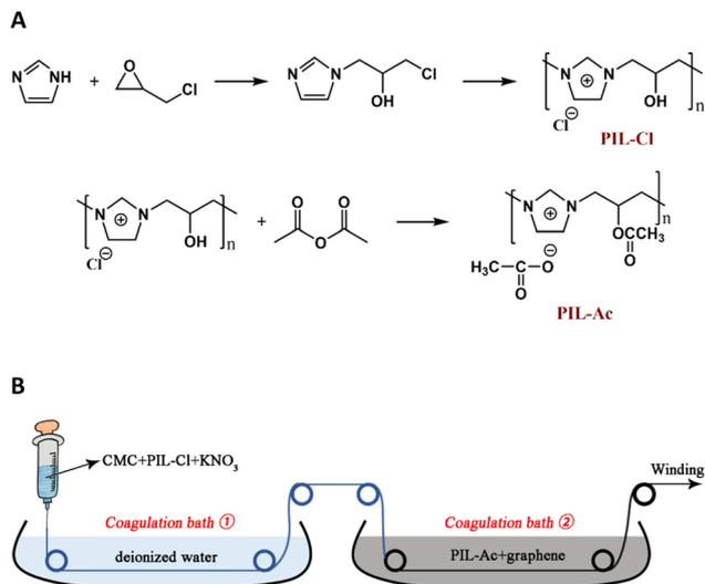
**Fig. 21** (A) The synthetic routes to PIL-Cl and PIL single bond Ac. (B) Preparation of graphene coated carboxymethyl cellulose (CMC) fibers. Reproduced from ref. 74 with permission from Elsevier, 2022.
