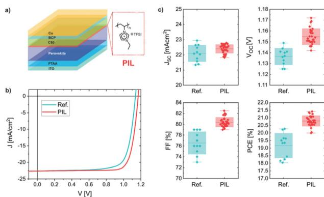
**Fig. 14** (a) Pin-type device layer architecture with the chemical structure of the poly(ionic liquid) (PIL) inserted between the perovskite and C60. (b) Typical current–voltage characteristic for a reference untreated cell and for a PIL-modified cell in reverse scan at  $0.025 \text{ V s}^{-1}$ . (c) Device parameter statistics for reference and the PIL-containing cells. Boxes indicate the standard deviation. Reproduced from ref. 42 with permission from The Royal Society of Chemistry, 2021.
