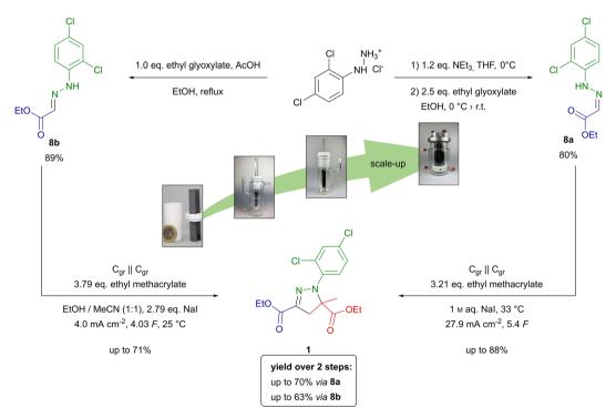
Scheme 2 Synthesis from screening to scale-up of mefenpyr-diethyl (1) from 2,4-dichlorophenylhydrazone hydrochloride via hydrazones 8a and
