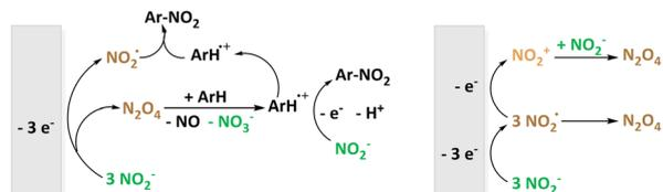
**Fig. 3** Electrochemical nitration using soluble  $\text{NO}_2^-$  as source of the nitrating agent according to the groups of Waldvogel (left) and Sereno (right).
