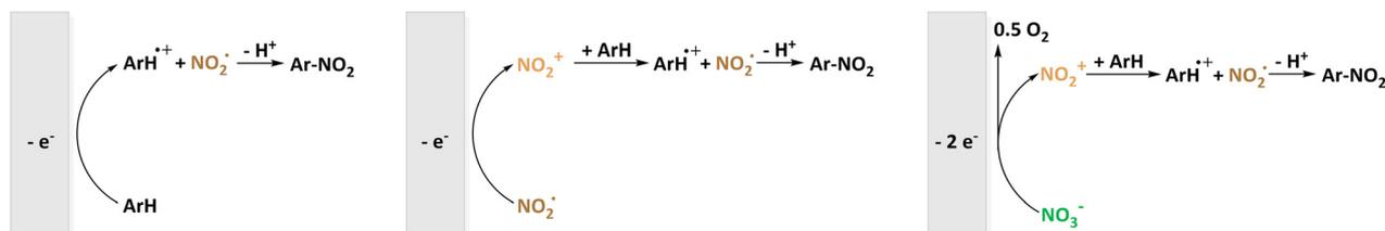
Fig. 2 Electrochemical nitration using  $\text{NO}_2^-$  as nitrating agent below (left) and above (middle) its potential of oxidation to  $\text{NO}_2^+$  and similarity to the reaction pathway using  $\text{NO}_3^-$  as source of  $\text{NO}_2^+$  (right).
