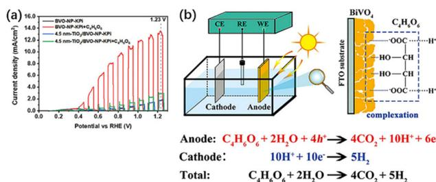
**Fig. 7** (a) Current density versus potential curves of BVO-NP and 4.5 nm  $\text{TiO}_2/\text{BVO-NP}$  photoanodes in potassium phosphate (KPi) and  $0.5 \text{ M C}_4\text{H}_6\text{O}_6$  solutions under AM 1.5G illumination or in the dark. (b) Schematic illustration of the detailed reaction process in the  $\text{BiVO}_4$  PEC fuel cell system. Adapted from ref. 58 with permission from John Wiley and Sons, copyright 2022.
