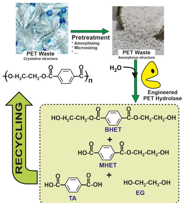
**Fig. 8** Schematic representation of a circular chemistry process for recovery and reuse of polyethyleneterephthalate (PET), based on the enzymatic hydrolysis by means of engineered biocatalysts.<sup>105</sup>
