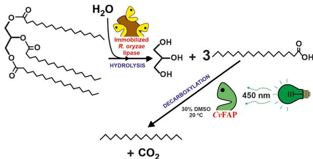
**Fig. 4** Two-steps biocatalytic cascade to transform natural triglycerides to alkanes by the consecutive actions of *Rhizopus oryzae* lipase, and the photoactivated fatty acid decarboxylase from *Chlorella variabilis* NC64A (CvFAP).<sup>30,31</sup>
