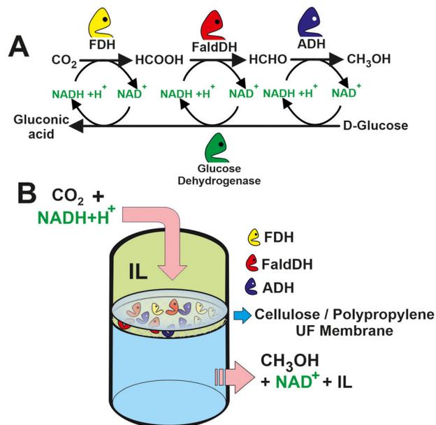
Fig. 6 (A) Scheme of a multi-enzyme system for methanol synthesis from CO<sub>2</sub> with *in situ* regeneration of NADH. (B) Set-up of the proposed IL-based multi-enzymatic membrane reactor for CO<sub>2</sub> transformation to methanol.<sup>80</sup>
