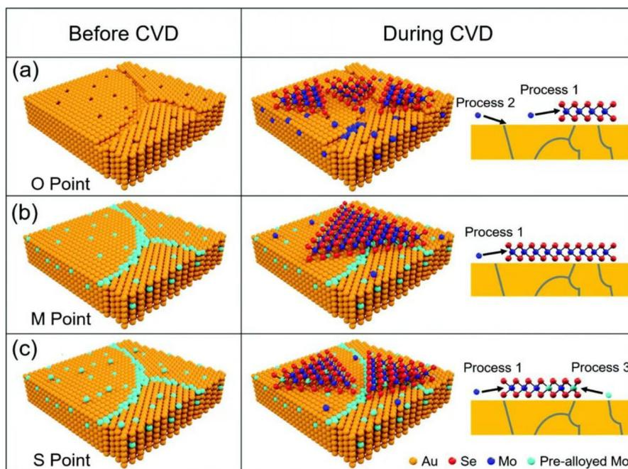
**Fig. 4** Schematic diagram of MoSe<sub>2</sub> growth on pre-alloyed Au with different Mo content. (a) The original polycrystalline Au surface with many defects, including vacancies and grain boundaries (b) Mo content got saturated at 900 °C. (c) Mo was oversaturated at 900 °C (reproduced from ref. 68 with permission from the Royal Society of Chemistry, copyright 2022).<sup>68</sup>
