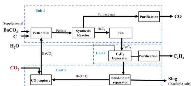
Fig. 7 Schematic diagram of the carbon-to-acetylene process with the co-production of carbon monoxide using BaC<sub>2</sub> as an intermediate.
