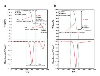
Fig. 2 Reaction behaviours of  $BaCO_3$  and C. (a) TG/DTG curves of a mixture of C/BaCO<sub>3</sub>. (b) TG/DTG curves of a mixture of C/CaCO<sub>3</sub>.
