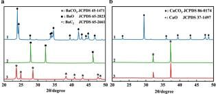
Fig. 4 XRD patterns of reactants and their corresponding products. (a) Ba system. (b) Ca system. (1) reactants and (2) heating products at 250 min (Ba system) and 325 min (Ca system), and (3) heating products at 600 min.
