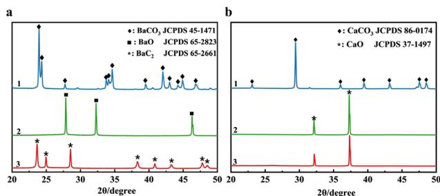
**Fig. 4** XRD patterns of reactants and their corresponding products. (a) Ba system. (b) Ca system. (1) reactants and (2) heating products at 250 min (Ba system) and 325 min (Ca system), and (3) heating products at 600 min.
