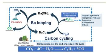
Fig. 8 Schematic of the barium-based carbon-to-acetylene process with the co-production of carbon monoxide.
