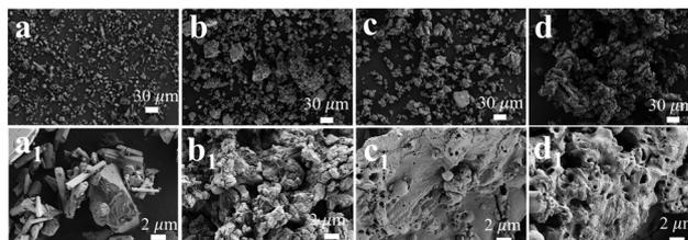
**Fig. 6** SEM images of the reactant and products: (a and a<sub>1</sub>) reactant and (b and b<sub>1</sub>) heating products at 1150 °C, (c and c<sub>1</sub>) at 1400 °C for 60 min, and (d and d<sub>1</sub>) at 1550 °C for 30 min.
