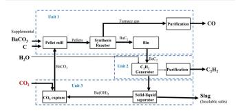
Fig. 7 Schematic diagram of the carbon-to-acetylene process with the co-production of carbon monoxide using  $BaC_2$  as an intermediate.
