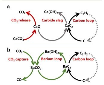
Fig. 1 Schematic of the carbon-to-acetylene process. (a) Calcium-based carbon-to-acetylene process. (b) Coupling process of carbon-to-acetylene with CO<sub>2</sub> capture based on Ba looping.
