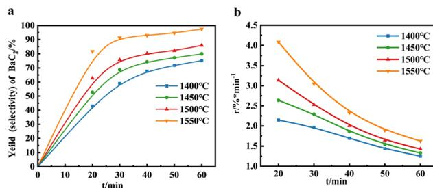
**Fig. 5** The effects of kinetic conditions on the formation of BaC<sub>2</sub>. (a) Dependence of the BaC<sub>2</sub> yield and Ba mass balance on the reaction temperature and time; (b) BaC<sub>2</sub> reaction rate dependence on the reaction temperature and time.
