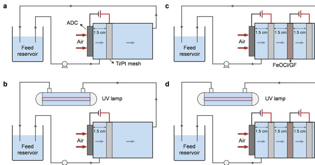
Fig. 1 Schematic illustration of different standalone or coupled degradation systems: (a) H<sub>2</sub>O<sub>2</sub>, (b) UV/H<sub>2</sub>O<sub>2</sub>, (c) HEF, and (d) HEF/UV.
