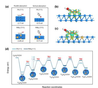
Fig. 6 (a) Different adsorption configurations on Pt(111) and PtRu(111). The charge density difference analysis of benzoic acid on (b) Pt(111) and (c) PtRu(111). The green and yellow colors substitute the charge accumulation and depletion regions, respectively. The isosurface level is all the same, equal to 0.03 e Å $^{-3}$ . (d) The relative energy diagram for the ECH of benzoic acid with the schematic top view of the corresponding reactants on the PtRu(111) surface.
