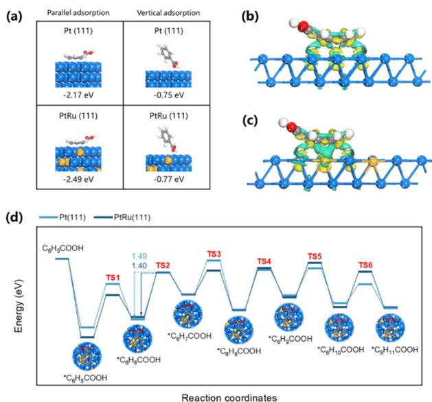
**Fig. 6** (a) Different adsorption configurations on Pt(111) and PtRu(111). The charge density difference analysis of benzoic acid on (b) Pt(111) and (c) PtRu(111). The green and yellow colors substitute the charge accumulation and depletion regions, respectively. The isosurface level is all the same, equal to  $0.03 e \text{ \AA}^{-3}$ . (d) The relative energy diagram for the ECH of benzoic acid with the schematic top view of the corresponding reactants on the PtRu(111) surface.
