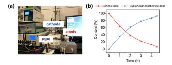
Fig. 8 (a) The photograph of the ECH electrolyzer cell and reaction system. (b) Relative content of benzoic acid and cyclohexanecarboxylic acid. Conditions: 0.2 M  $\rm H_2SO_4$ , 10 mM benzoic acid,  $\rm -100$  mA, room temperature.
