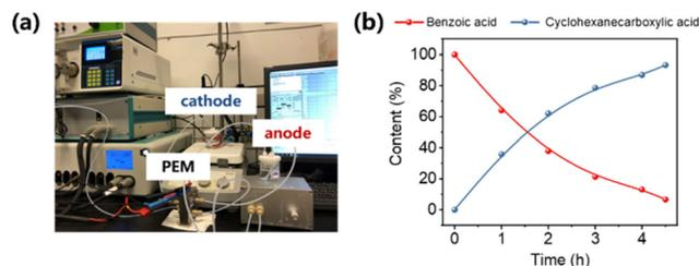
**Fig. 8** (a) The photograph of the ECH electrolyzer cell and reaction system. (b) Relative content of benzoic acid and cyclohexanecarboxylic acid. Conditions: 0.2 M  $\text{H}_2\text{SO}_4$ , 10 mM benzoic acid,  $-100$  mA, room temperature.
