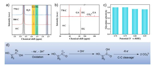
Fig. 4 (a)  $^{1}$ H NMR and (b)  $^{13}$ C NMR spectra of the electrolyte at different Coulomb quantities. (c) Electro-oxidation selectivity of EG to glycolate at different voltages. (d) Reaction pathways of EG electro-oxidation on Pd<sub>1</sub>Ag<sub>1</sub> NPs.
