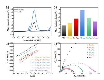
Fig. 2 (a) CVs of Pd<sub>1</sub>Ag<sub>1</sub> NPs and commercial Pd/C in 1 M KOH and 1 M EG solution at 10 mVs<sup>-1</sup>; (b) comparison of peak mass currents of Pd<sub>x</sub>Ag<sub>v</sub> NPs and commercial Pd/C; (c) Tafel slope plots and (d) Nyquist plots of  $Pd_xAg_y$  NP samples and commercial Pd/C in 1 M KOH containing 1 M EG.
