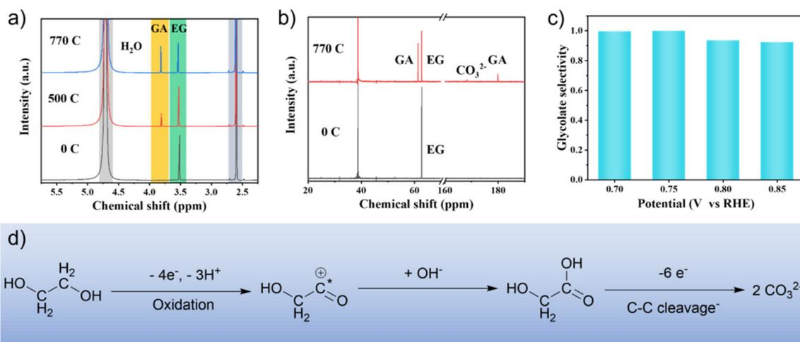
**Fig. 4** (a) <sup>1</sup>H NMR and (b) <sup>13</sup>C NMR spectra of the electrolyte at different Coulomb quantities. (c) Electro-oxidation selectivity of EG to glycolate at different voltages. (d) Reaction pathways of EG electro-oxidation on Pd<sub>1</sub>Ag<sub>1</sub> NPs.
