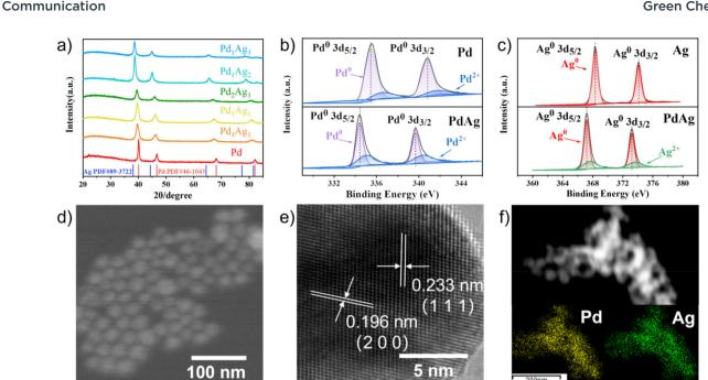
Fig. 1 (a) XRD patterns of Pd<sub>x</sub>Ag<sub>v</sub> NPs. High-resolution XPS spectra of (b) Pd 3d and (c) Ag 3d. (d) SEM, (e) HRTEM and (f) mapping images of Pd<sub>1</sub>Ag<sub>1</sub> NPs
