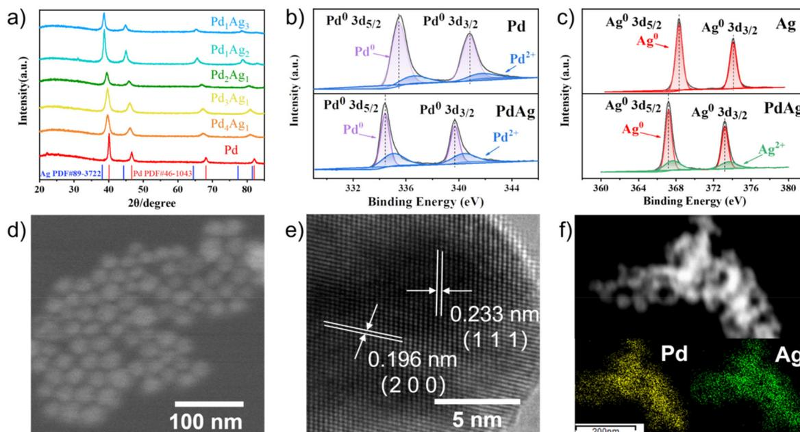
**Fig. 1** (a) XRD patterns of Pd<sub>x</sub>Ag<sub>y</sub> NPs. High-resolution XPS spectra of (b) Pd 3d and (c) Ag 3d. (d) SEM, (e) HRTEM and (f) mapping images of Pd<sub>1</sub>Ag<sub>1</sub> NPs.
