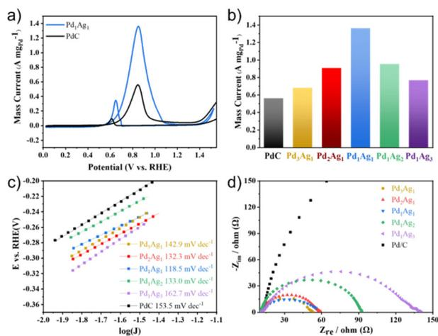
**Fig. 2** (a) CVs of Pd<sub>1</sub>Ag<sub>1</sub> NPs and commercial Pd/C in 1 M KOH and 1 M EG solution at 10 mVs<sup>-1</sup>; (b) comparison of peak mass currents of Pd<sub>x</sub>Ag<sub>y</sub> NPs and commercial Pd/C; (c) Tafel slope plots and (d) Nyquist plots of Pd<sub>x</sub>Ag<sub>y</sub> NP samples and commercial Pd/C in 1 M KOH containing 1 M EG.
