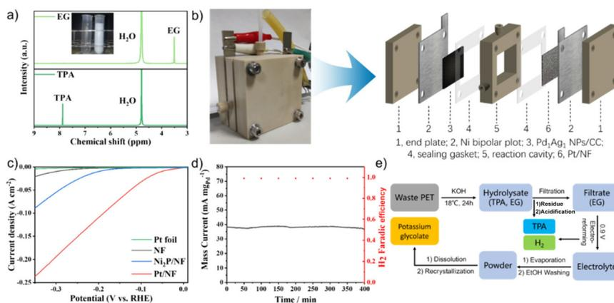
**Fig. 5** (a) <sup>1</sup>H NMR spectra of the hydrolysate and TPA from green plastic bottles. Inset: images of the hydrolysate and TPA powder. (b) Images and schematic of a two-electrode flow cell reactor. (c) HER linear sweep voltammety curves for various materials in PET hydrolysates. (d) *I*–*T* curves and faradaic efficiency of H<sub>2</sub> of waste PET plastic hydrolysate in a flow cell reactor. (e) Schematic of electro-reforming of PET and product separation.
