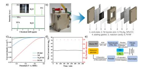
Fig. 5 (a) <sup>1</sup>H NMR spectra of the hydrolysate and TPA from green plastic bottles. Inset: images of the hydrolysate and TPA powder. (b) Images and schematic of a two-electrode flow cell reactor. (c) HER linear sweep voltammetry curves for various materials in PET hydrolysates. (d) I-T curves and faradaic efficiency of H<sub>2</sub> of waste PET plastic hydrolysate in a flow cell reactor. (e) Schematic of electro-reforming of PET and product separation.
