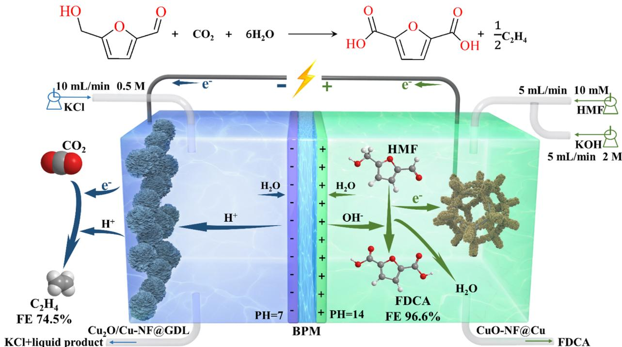
Fig. 1 Schematic illustration of integrated electrolysis flow cell coupling CO<sub>2</sub>RR with HMFOR.
