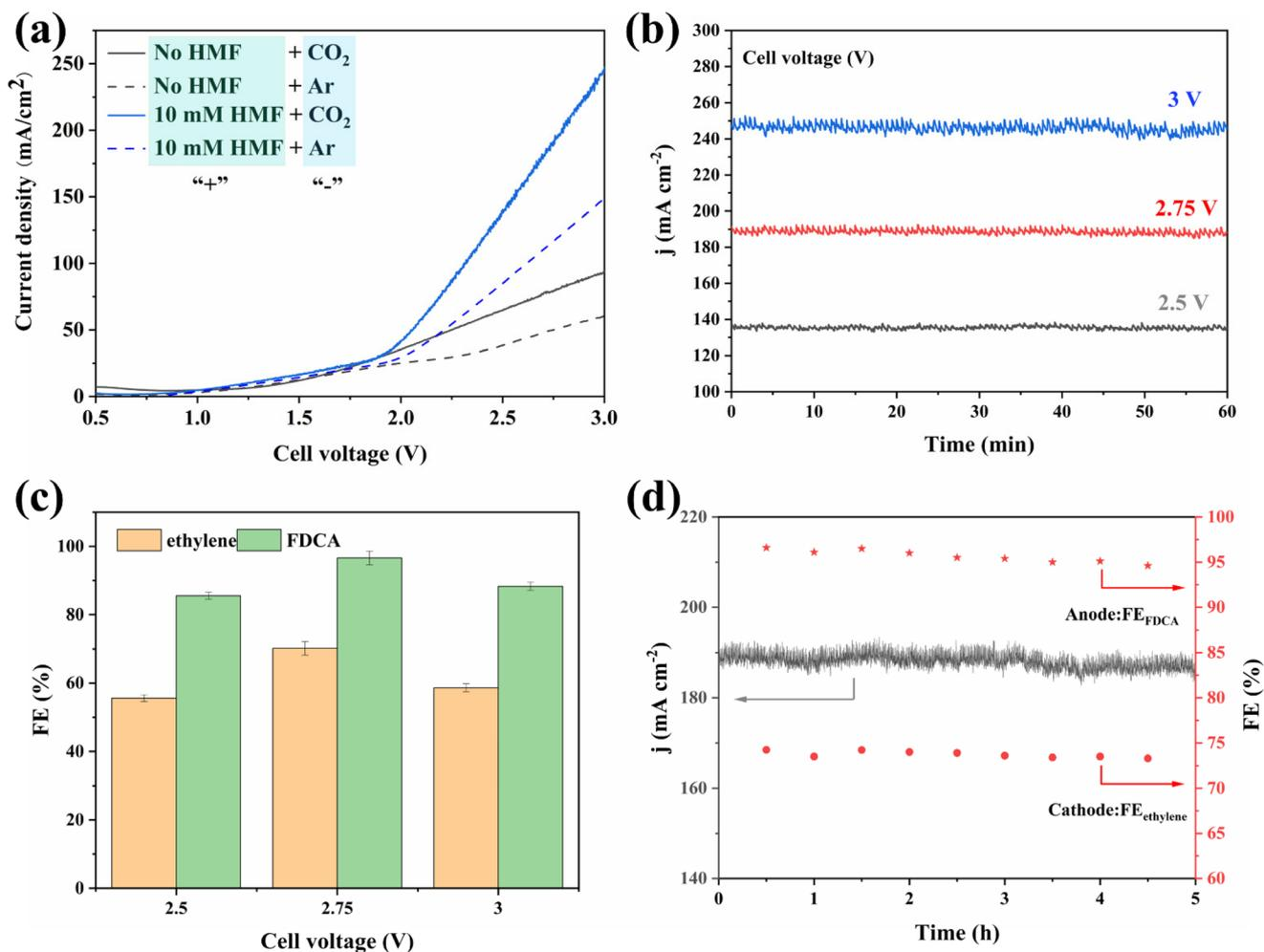
Fig. 8 (a) LSV curves recorded in two-electrode setup. "+": anodic compartment; "-": cathodic compartment. (b) Chronoamperometry curves under different cell voltages, (c) corresponding FE for CO<sub>2</sub>RR-HMFOR couple under different cell voltages, (d) stability test of Cu-based nanoflower sheets in CO<sub>2</sub>RR-HMFOR coupled reaction under a cell voltage of 2.75 V.
