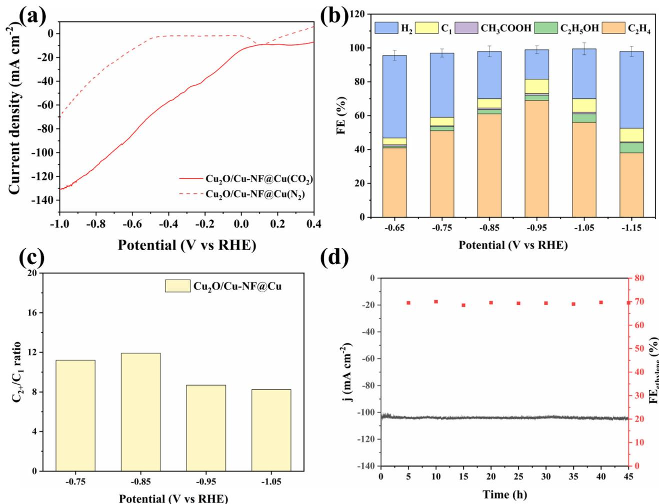
Fig. 5 (a) LSV curves over Cu<sub>2</sub>O/Cu-NF@Cu in Ar and CO<sub>2</sub> saturated KCl electrolyte, (b) FEs of products over Cu<sub>2</sub>O/Cu-NF@Cu, (c) C<sub>2</sub><sup>+</sup>/C<sub>1</sub> ratios for CO<sub>2</sub>RR products, (d) long-term stability test of 45 h at -0.95 V vs. RHE for Cu<sub>2</sub>O/Cu-NF@Cu.
