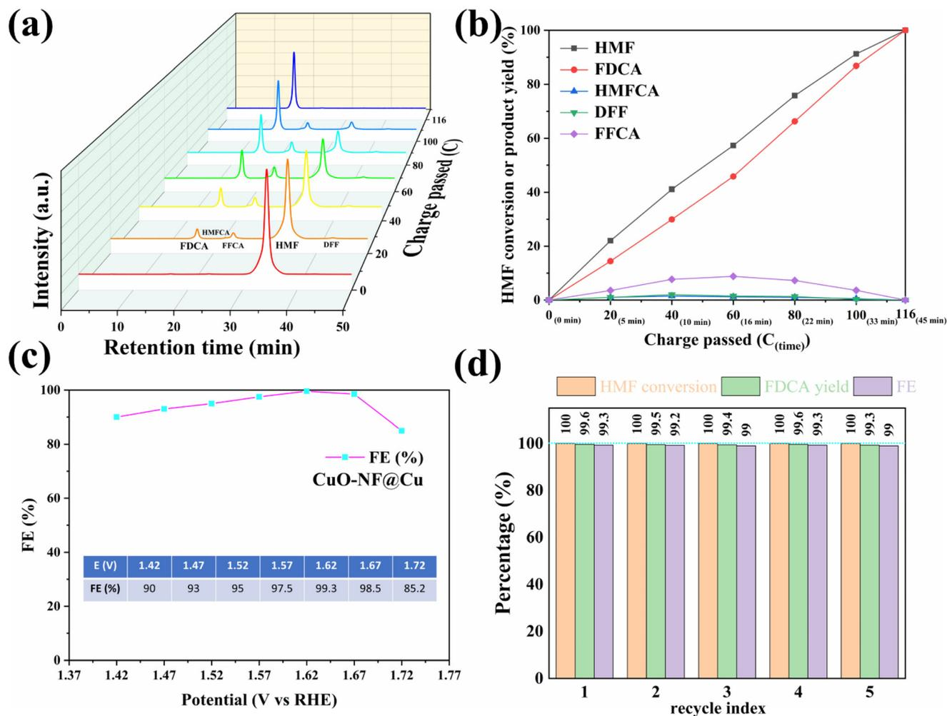
**Fig. 6** (a) HPLC spectra of HMF reaction solution vs. passed charges during reaction, (b) HMF conversion and products yields vs. passed charges during reaction, (c) FE of FDCA at varied potentials, (d) recycling tests of CuO-NF@Cu.
