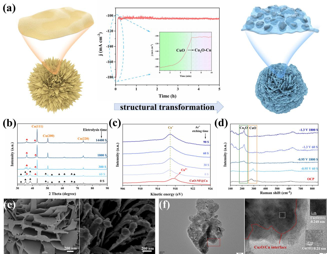
**Fig. 4** (a) Schematic illustration of morphology changes during the electrochemical reduction of CuO-NF@Cu, (b) XRD patterns of CuO-NF@Cu at different reduction times, (c) Cu LMM Auger spectra of CuO-NF@Cu and Cu<sub>2</sub>O/Cu-NF@Cu with different Ar<sup>+</sup> etching times, (d) *in situ* Raman spectra of Cu<sub>2</sub>O/Cu-NF@Cu in different conditions, (e) SEM images of fresh CuO-NF@Cu and Cu<sub>2</sub>O/Cu-NF@Cu, (f) TEM and HRTEM images of Cu<sub>2</sub>O/Cu-NF@Cu.
